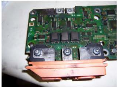
Control Board Only Collateral Damage / Sooted
