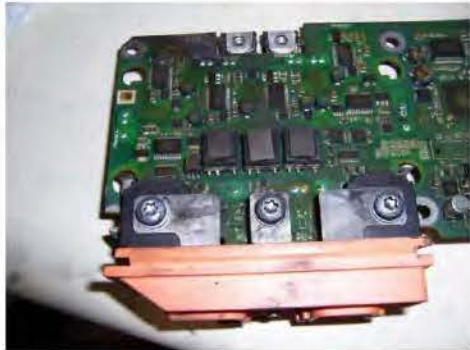
Control Board Only Collateral Damage / Sooted
