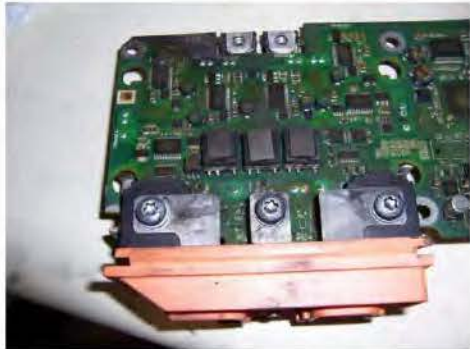
Control Board Only Collateral Damage / Sooted
