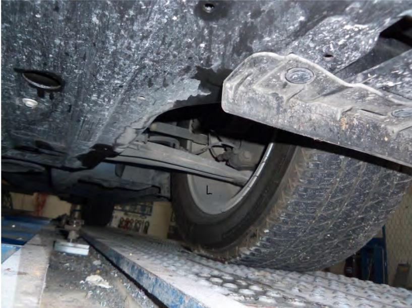
A photograph showing the left front suspension system of a vehicle. The view is from underneath the car, showing the control arm, steering knuckle, and tire. A white 'L' is marked on the tire. The suspension components appear to be in good condition. | No              |
