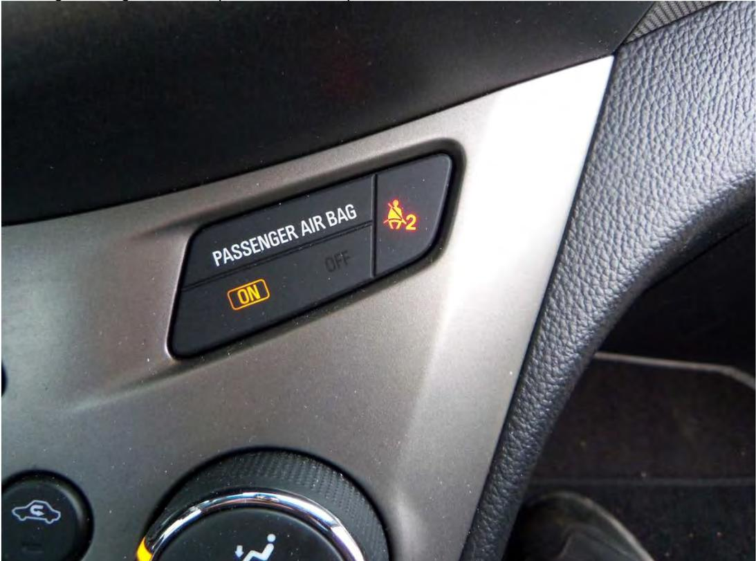
A close-up photograph of the passenger airbag control panel, similar to the previous one. In this image, the word 'ON' is illuminated in yellow, and the airbag icon (a person with arms outstretched) is also illuminated in yellow. The 'OFF' text and the red 'X' icon are not lit.                                                                                                                                                                                        | No              |
