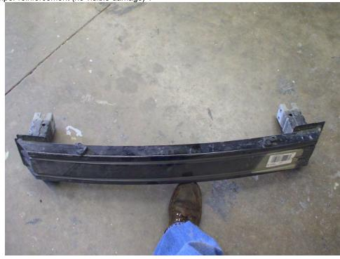
26 Front bumper reinforcement (no visible damage) 2
