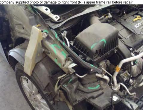
22 Close-up of buckle in RF frame rail
