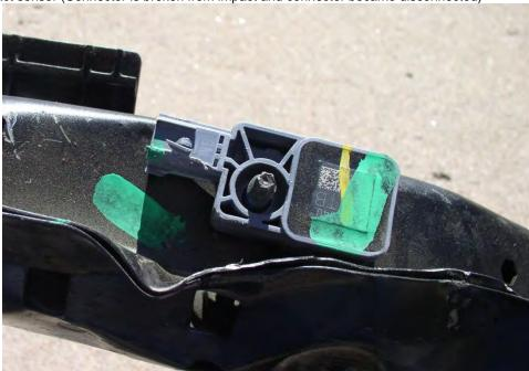
Right impact sensor connector view showing lock is still in locked position
