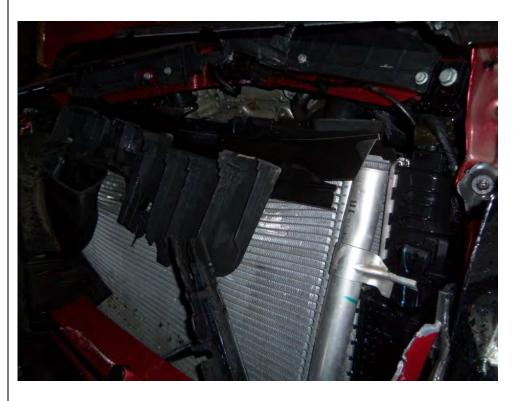
36 Piece Missing from Front Bumper Reinforcement
