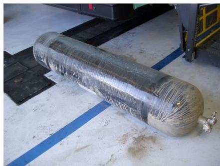
Dislodged tank from bus #2014
