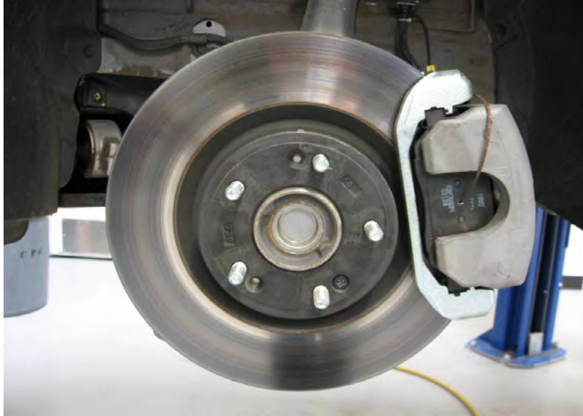
THERMOCOUPLE INSTALLATION OF LEFT FRONT
