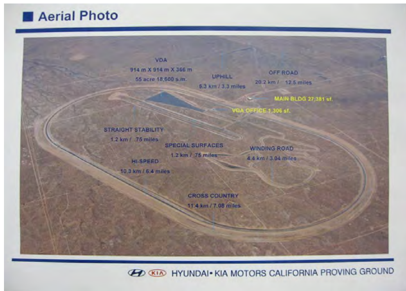
TEST TRACK DIMENSIONED LAY-OUT
