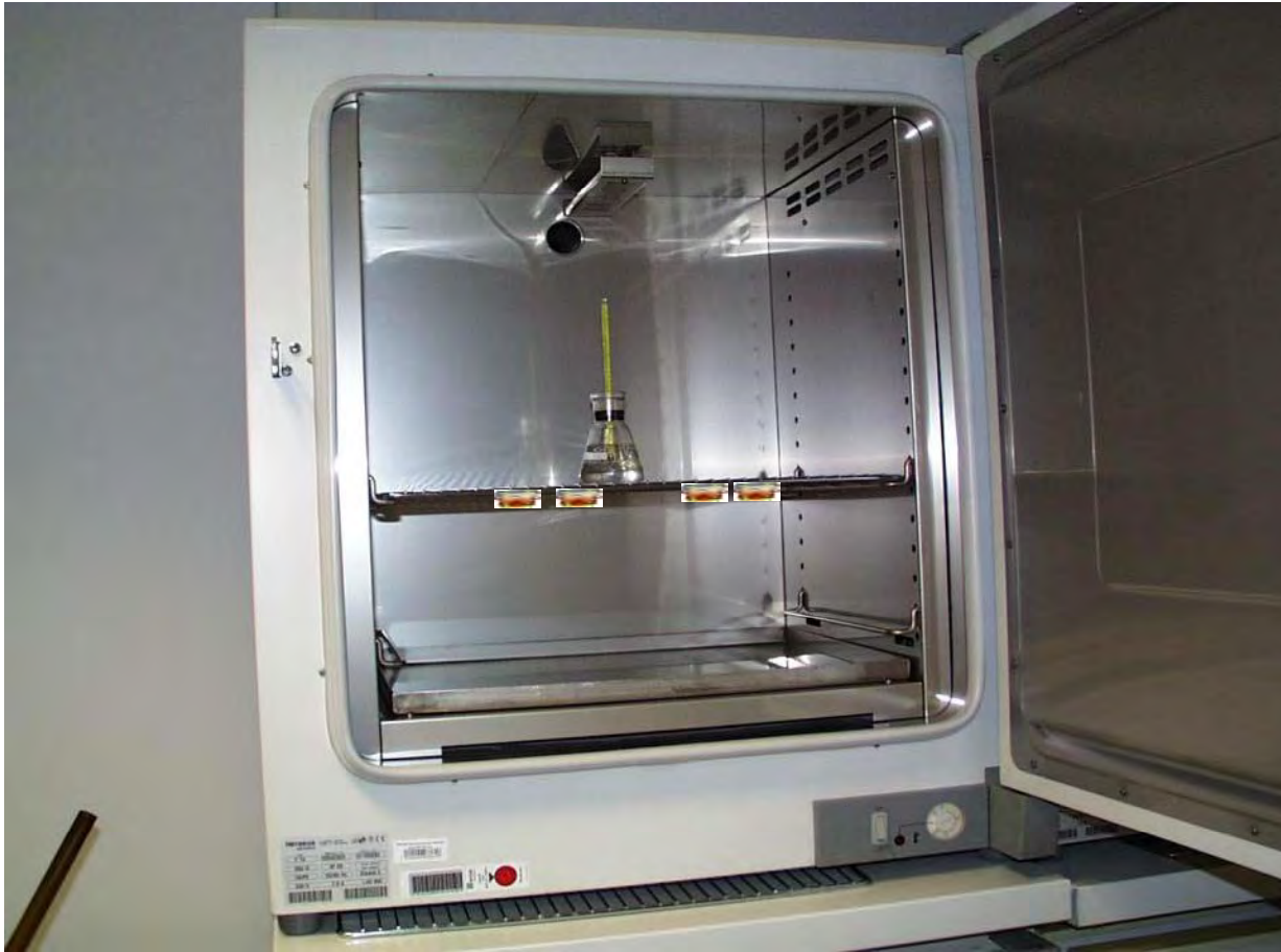
Picture of opened convection oven with petri dishes and thermometer-equipped silicone oil flask ((metal tablet is omitted for clarity)
