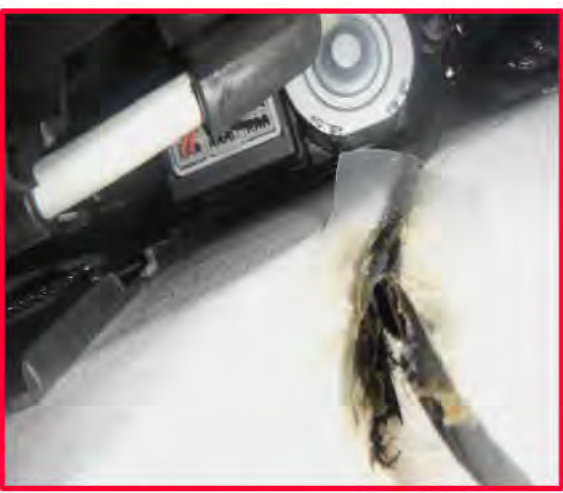
Sun visor screw shorted the wiring on the passenger side
