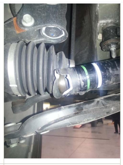
Found right side axle broken. No other damage was done. Axle part number: 49501-2W600
