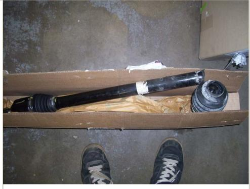
The weld on the end of the axle shaft appears to have poor penatration of the metal.
