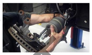
11. If the axle does not come free with a tug as in step 10, utilize a pry bar and gently dislodge the axle from the transmission.
