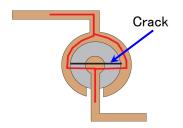
The shape of the resistance was changed from the rectangle to the circle in order to improve the tolerance in occurring a crack.
