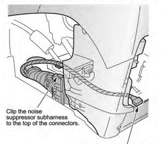
Route the noise suppressor subharness through the console front opening.
