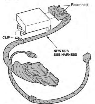
Reinstall the SRS unit and SRS subharness into the vehicle and install the three Torx bolts fingertight.
