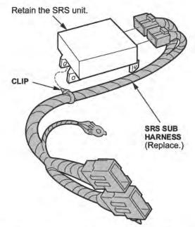
12. Cut the connector off one end of the SRS subharness to make sure that it cannot be reused.
