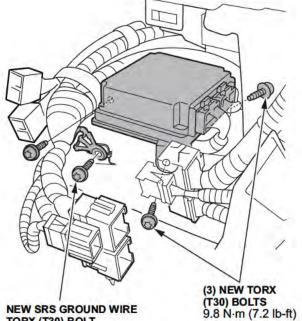
TORX (T30) BOLT 9.8 N·m (7.2 lb-ft) 13. Install the subharness and noise suppressor.
