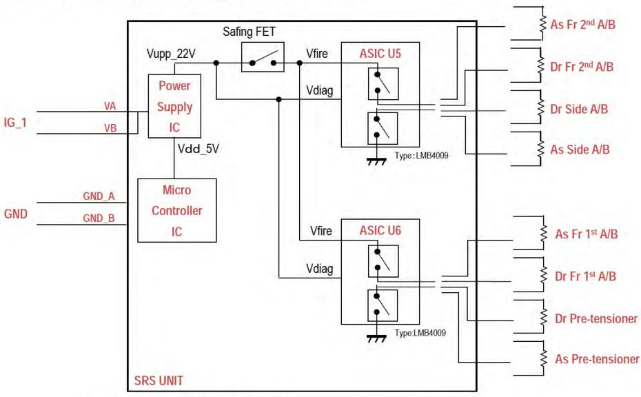
Micro Controller IC controls SW in each FET.
