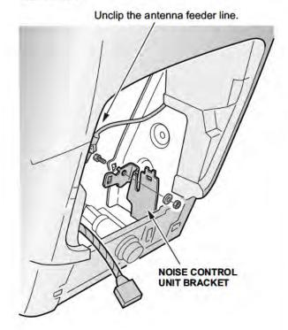
20. Connect the connector to the noise suppressor.
