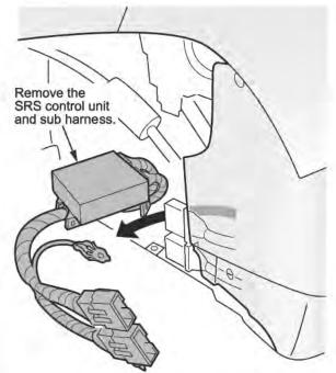
Remove the subharness clip from the underside of the SRS unit, then disconnect the subharness from the unit.
