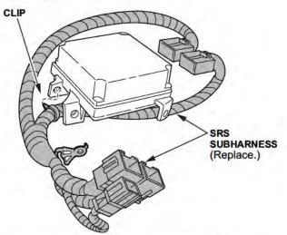
10. Cut the connector off one end of the SRS subharness to make sure that it cannot be reused.
