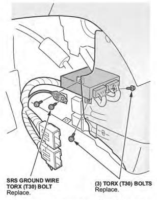
9. Remove the SRS ground wire Torx (T30) bolt.
