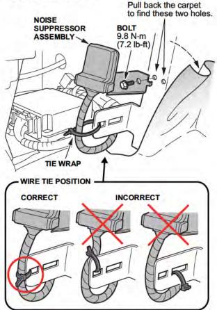
Install a tie wrap as shown to hold the suppressor subharness in place. Make sure that the SRS subharness does not interfere with or rub on the shift cable.
