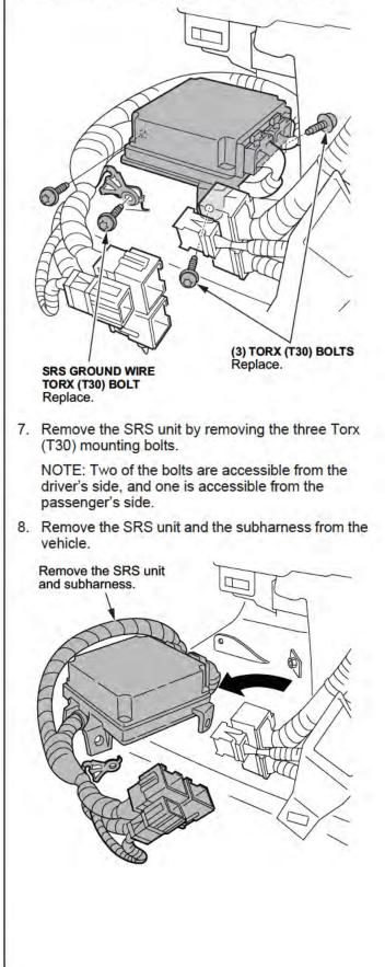
9. Remove the subharness clip from the underside of the SRS unit, then disconnect the subharness from the unit.
