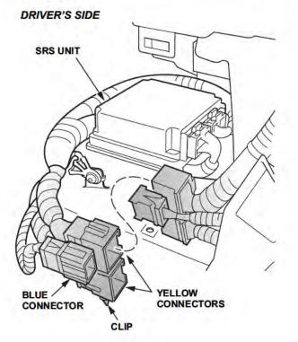
6. Remove the SRS ground wire Torx (T30) bolt.
