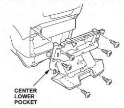
Remove the driver's and passenger's heater lower covers.
