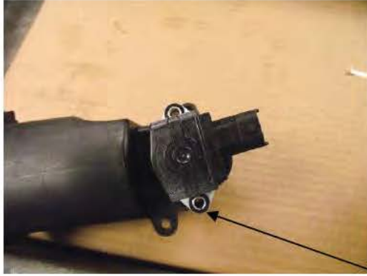
Need 2 screws/muffler for the muffler fitting, 10 screws total
