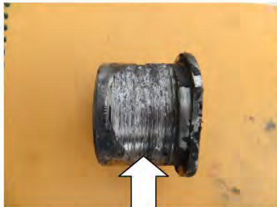
Worn Pulley Pin
