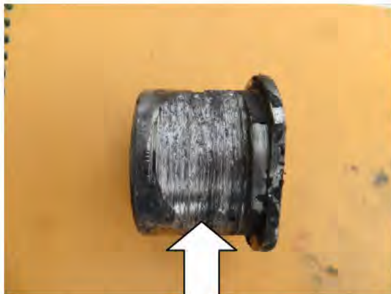
Worn Pulley Pin
