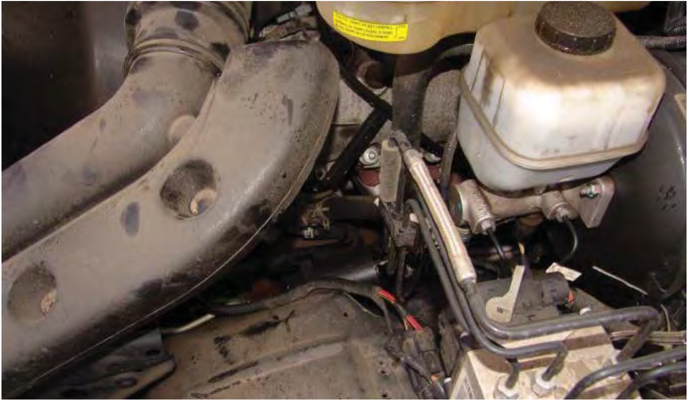
Photograph013.JPG: Brake fluid reservoir.
