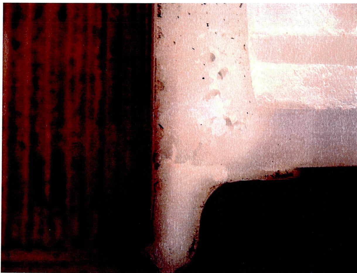
Voids in polymer created by poor polymer processing. Fracture of rim.
