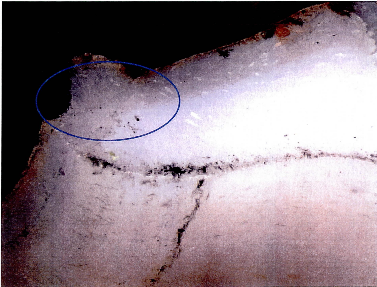
Cracks at insert groove.
