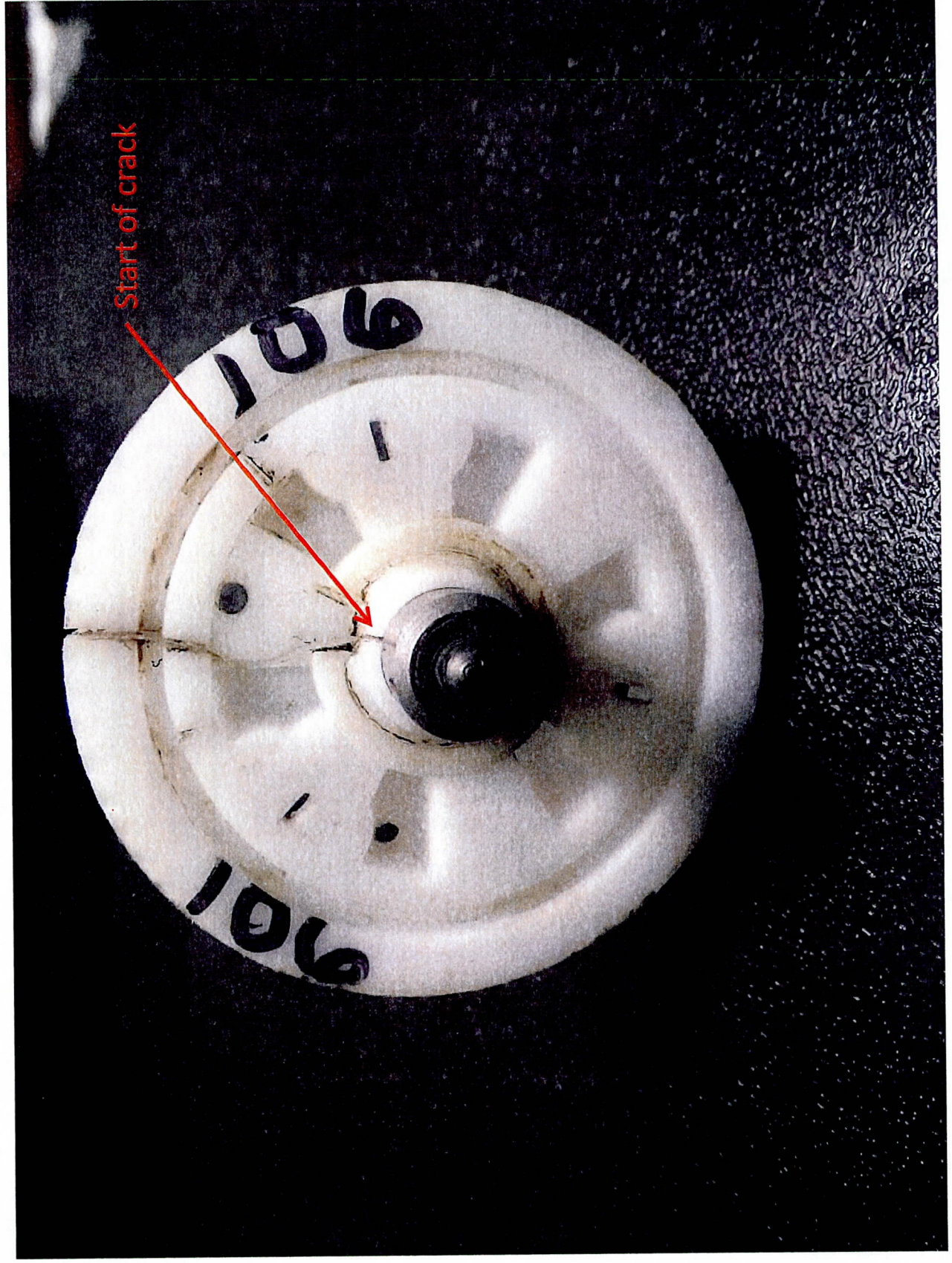
Typical cracked gear
