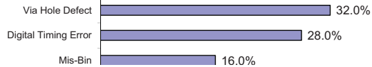
9L8E Warranty Return Summary, Model Years 2009-2010 DTC's P0122 & P0222, Excluding P2135 No DTC Code And In-Process Returns Omitted
