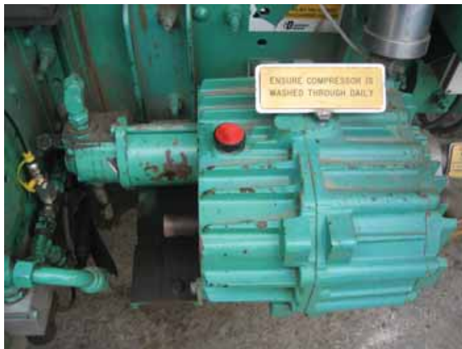
Figure 2 Roots compressor, driven from a gearbox PTO.
