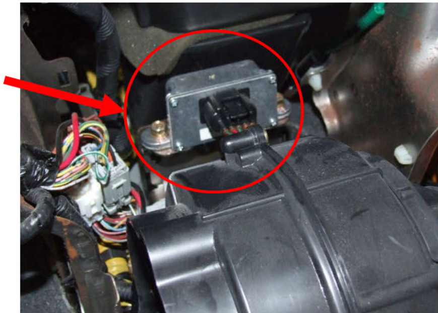
Yaw rate sensor as mounted in the vehicle center counsel.
