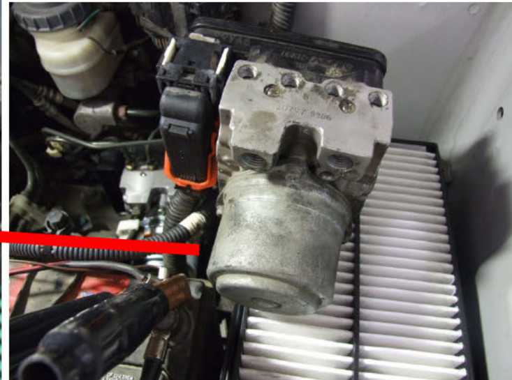
Vehicle Stability Assist Modulator With brake lines removed.
