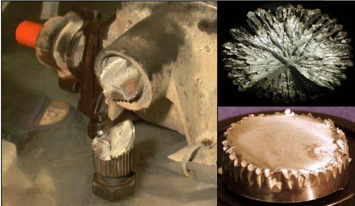
Figure 3. Steering gear sector shaft overload failure (left), MY1999-2001 Ford F-Series Super Duty, EA01-009. Sector shaft fracture surface for fatigue failure (upper right) and overload failure (lower right).
