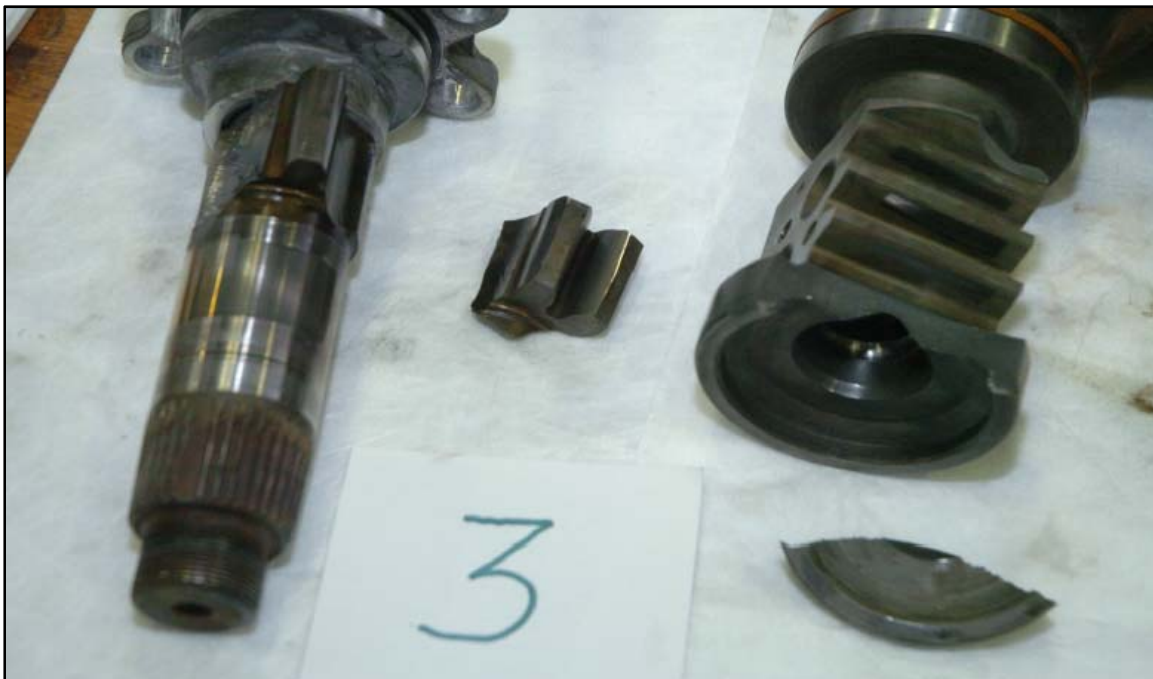
Figure 4. Steering gear teeth fracture overload failure, MY 2005-09 Ford F-Series Super Duty (PE13-014).
