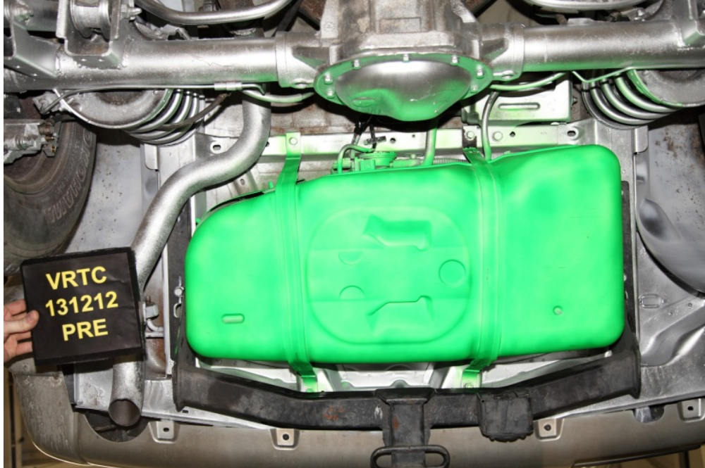
Figure 28 - Test #8 Pre-test target vehicle fuel tank close-up view
