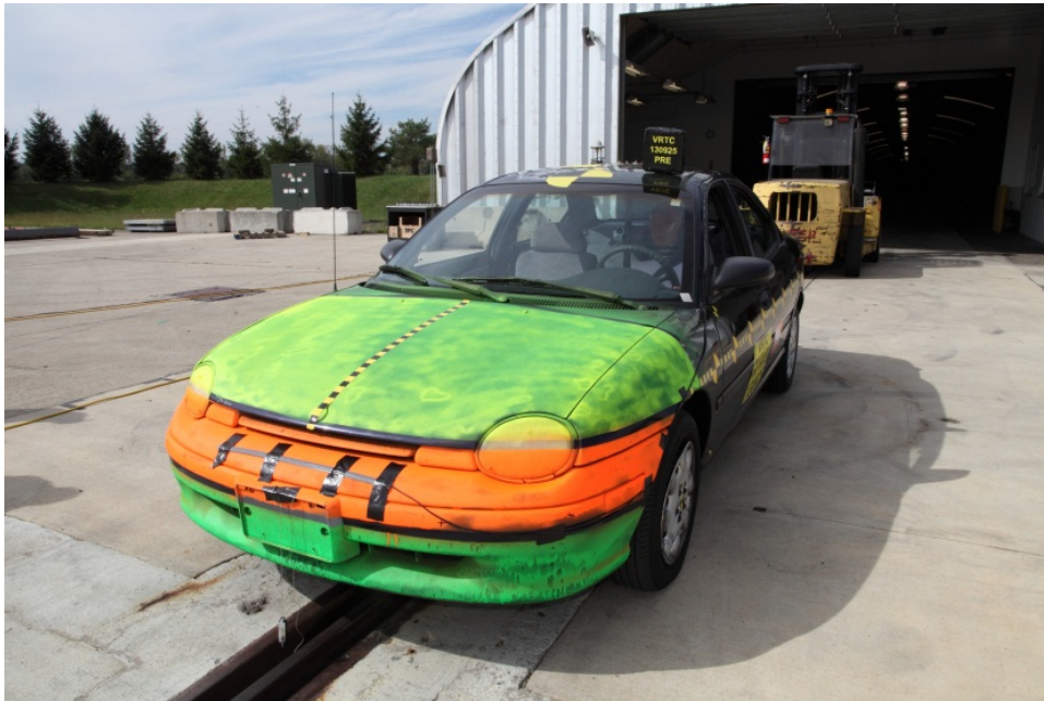
Figure 5 - 1997 Plymouth Neon bullet vehicle with painted regions
