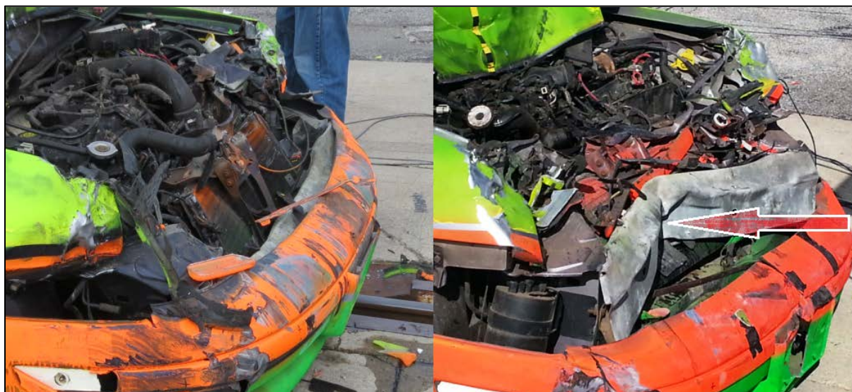
Figure 7 - Neon bumper reinforcement Test 1 vs. Test 2. Arrow at hitch-receiver contact
