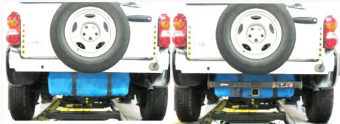
Figure 2 - Jeep Liberty without hitch-receiver and with hitch-receiver installed
