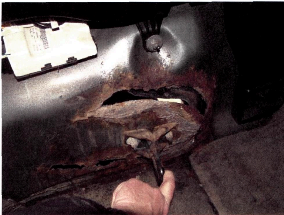
Figure 7 – Severe Corrosion on VOQ Vehicle
