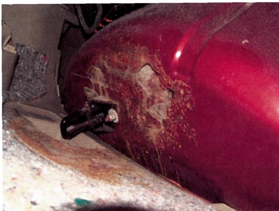
Figure 9 – Partially Corroded Seat Anchor
