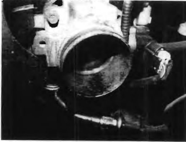
14. A view indicating the throttle blade is closed.
