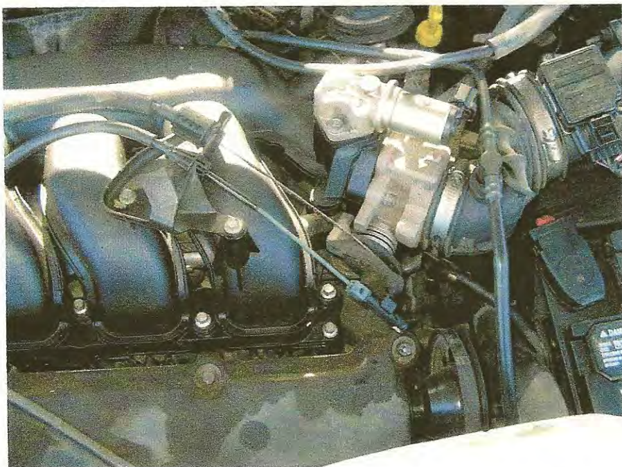
PLATE 5 : Looking down on the front of the engine and the accelerator cable and cruise control cable together at the throttle.
