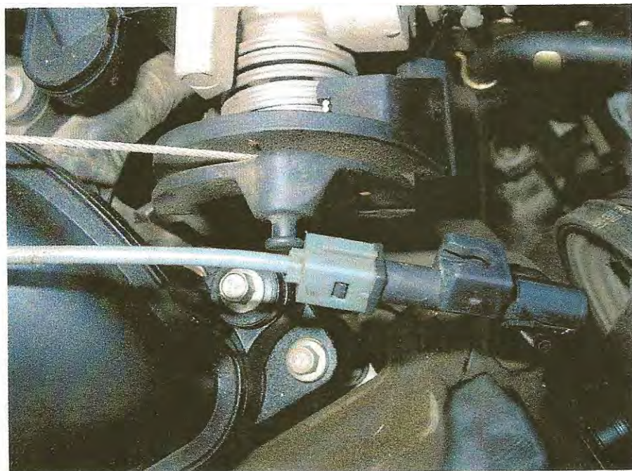
PLATE 8 : The throttle button is hung on the cruise control connector further up, on the latter than in the view above, holding the throttle open even further.
