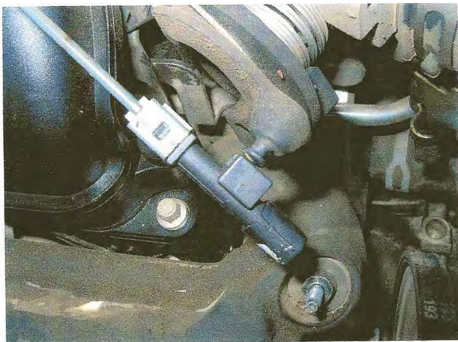
PLATE 6 : The end of the cruise control cable and connector (nearest the camera), which is not secured to the button on the throttle which opens by movement to the left.
