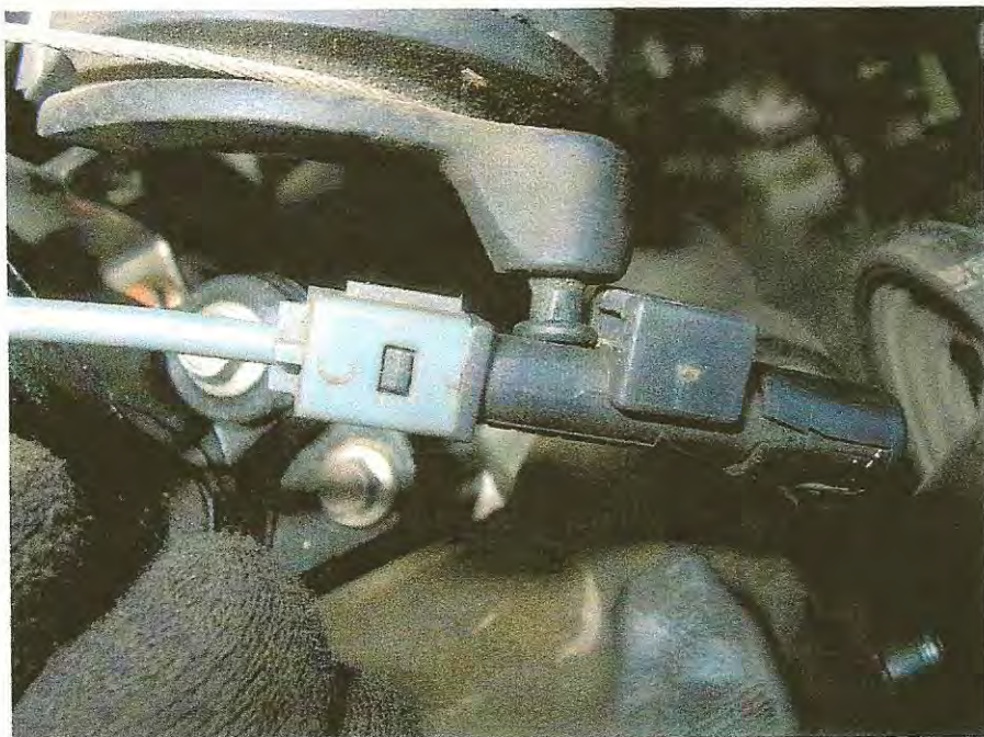
PLATE 7 : The cruise control connector body is supporting the throttle connector button, preventing the throttle from closing.
