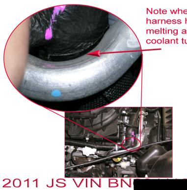
Note where the harness had been melting against the coolant tube
