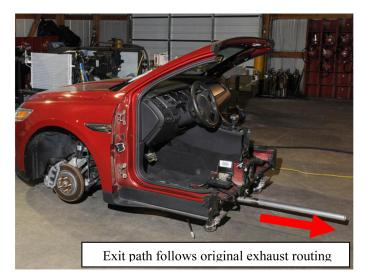
Figure E. Exit Path for Heated Exhaust
