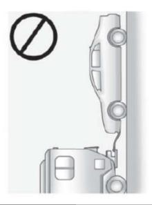
Notice: If the vehicle is towed with all four wheels on the ground, the drivetrain components could be damaged.
