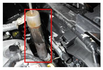
Figure D. Heat Tube and Top Cap.
