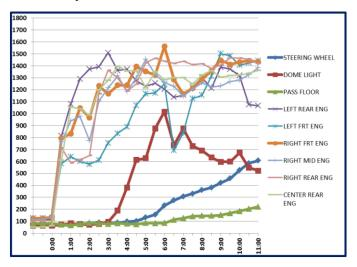
Figure T. R1234yf Temperature v. Time Plot (F° on the vertical axis; Time in minutes on the horizontal axis)
