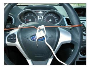
Figure M. Thermocouple 1 at Steering Wheel
