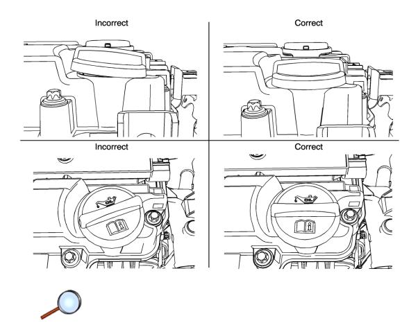
**Note:** Oil fill cap must be properly seated and tightened during installation.
