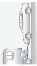
To dinghy tow the vehicle from the front with all four wheels on the ground:
