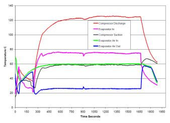
Figure G. A/C System Operation during Testing
