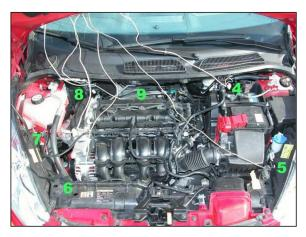
Figure P. Thermocouples 4 - 9 at Various Engine Compartment Locations
