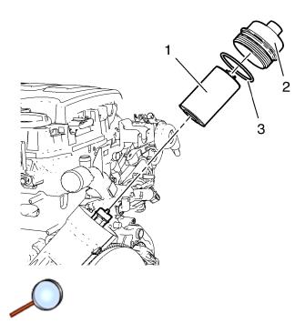
Note: Lubricate the NEW oil filter cap seal ring with engine oil.
