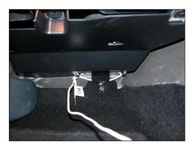
Figure O. Thermocouple 3 in Passenger Foot Well
