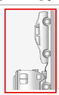
To dinghy tow the vehicle from the front with all four wheels on the ground:
