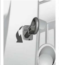
Screw in the towing eye as far as it will go until it stops in a horizontal position.
