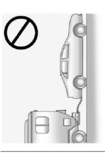
Notice: Towing the vehicle from the rear could damage it. Also, repairs would not be covered by the vehicle warranty. Never have the vehicle towed from the rear.
