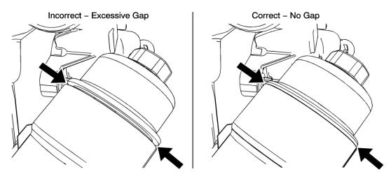
**Caution:** Ensure oil filter cap is completely seated on oil filter housing. If not completely seated an oil leak may occur.
