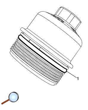
**Note:** Clean oil filter cap and lubricate the NEW oil filter cap seal ring with clean engine oil. Ensure oil filter cap seal ring is in proper position as shown.
