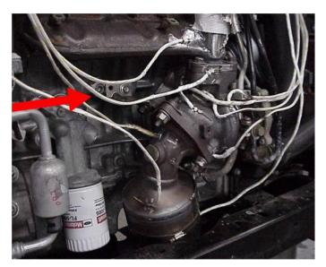
Figure B. Thermocouples (Heat Shield Removed)
