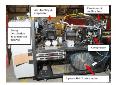
Figure F. Identification of A/C Test Stand Components
