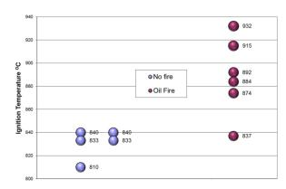
Figure I. R134a Testing Results
