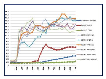
Figure S. R134a Temperature v. Time Plot (F° on the vertical axis; Time in minutes on the horizontal axis)
