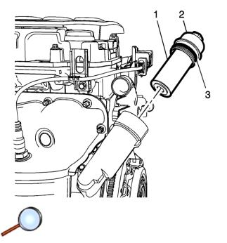
6. Install the engine oil filter cap (2) with NEW engine oil filter cap seal ring (3) and NEW oil filter element (1) hand tight.
