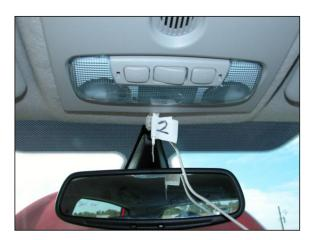
Figure N. Thermocouple 2 Centered, Near Dome Light
