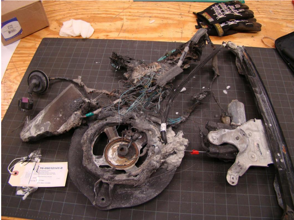
Photograph 1 The internal electrical door components.
