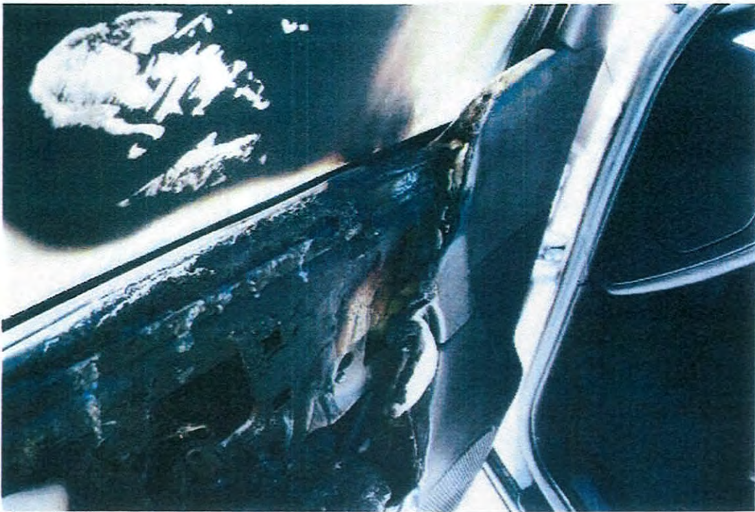
Photo #16 Views the area of origin on the driver's door
