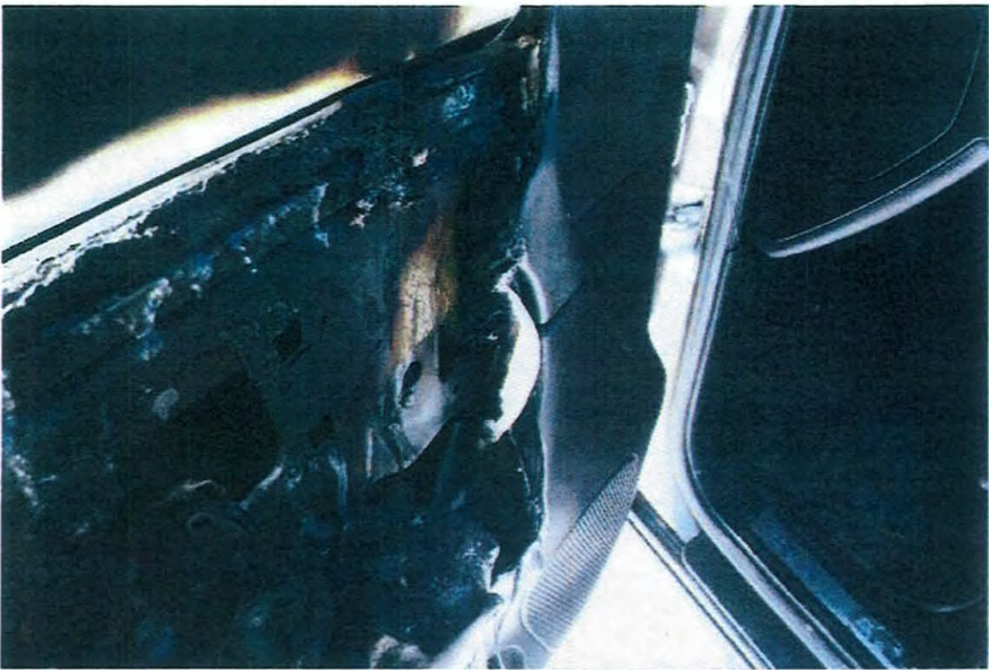
Photo #14 Views the burn pattern at the driver's door
