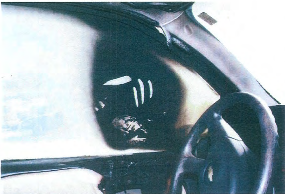
Photo #18 Views the burn pattern on the head liner
