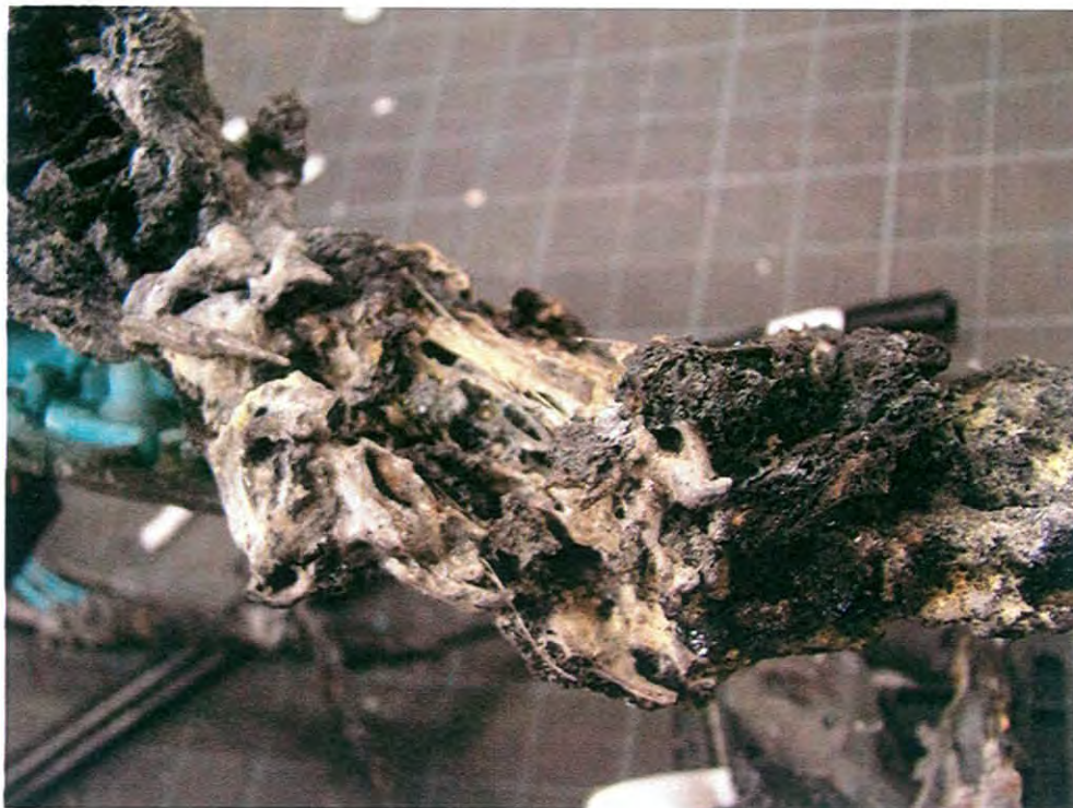
Photograph 6 It is possible that the origin of the fire lies within the melted components or that the evidence was consumed in the fire.
