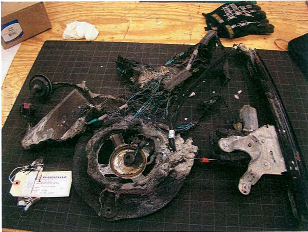
Photograph 1 The internal electrical door components.
