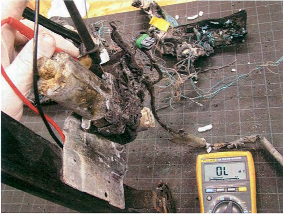
Photograph 3 No shorts to ground were found in the motor.
