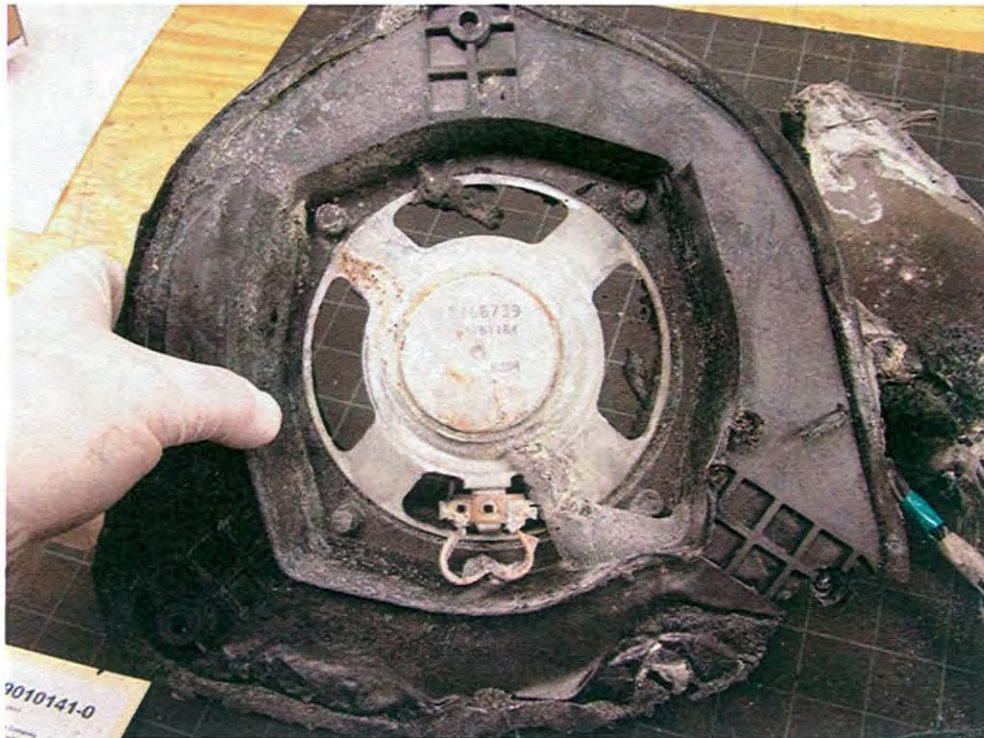
Photograph 4 The speaker damage appears to be located away from the wiring.
