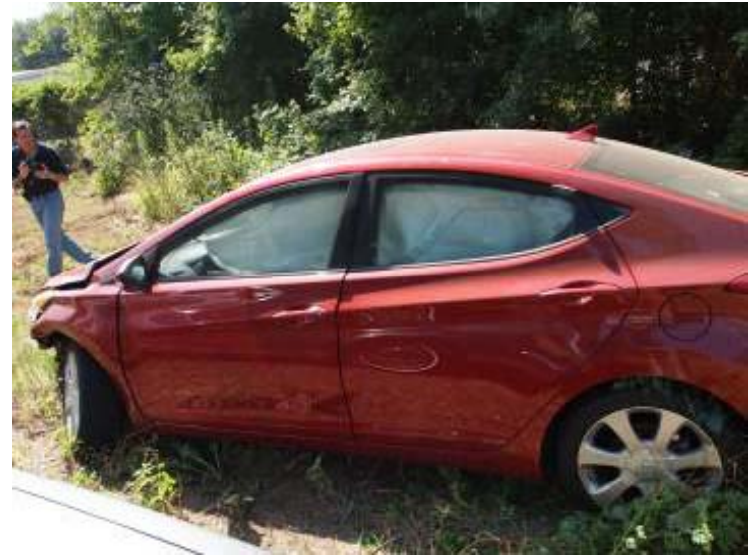
There is no LH SIDE door and left side body damage
