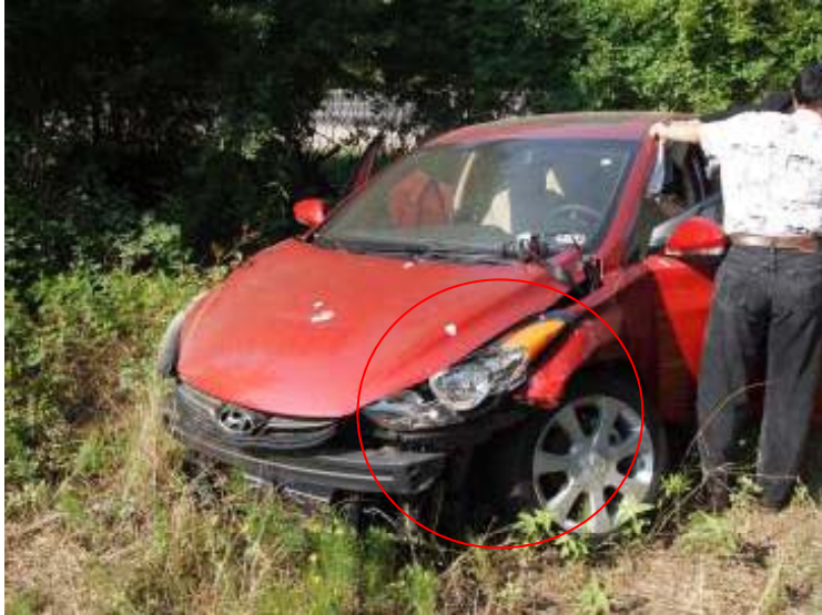
→ Accident circumstance detail verification anticipation (with HMA) From left side impact form, hood/fender/tire area deformation occurrence
