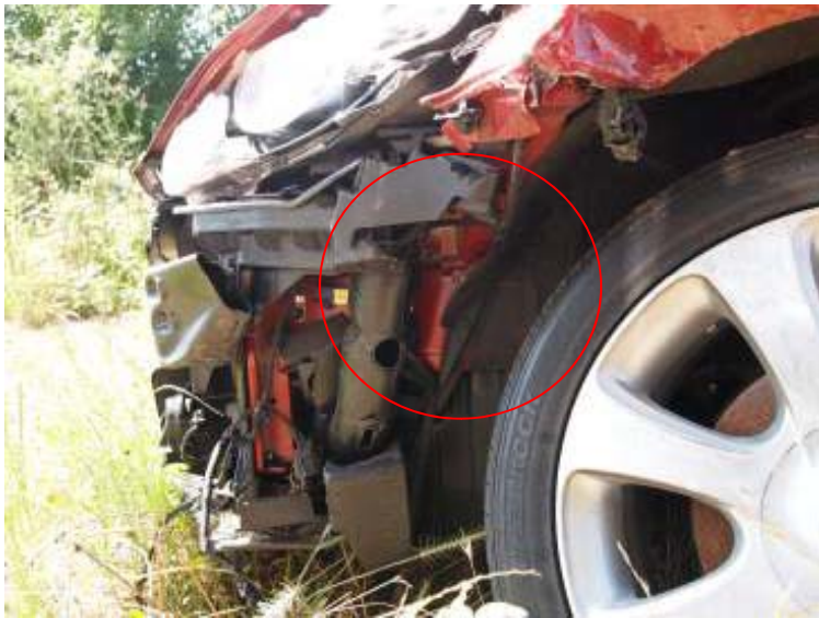
Body deformation area detailed photo-S/MBR mid part bending occurs
