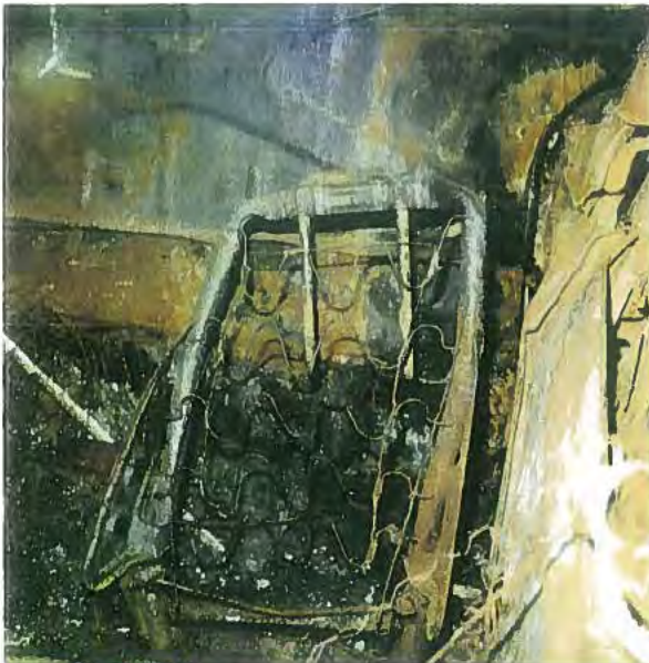
DRIVER SEAT TOP 3 SPRINGS DEF FORWARD BOTTOM 2 SPRINGS DEF RWD - PL-03
