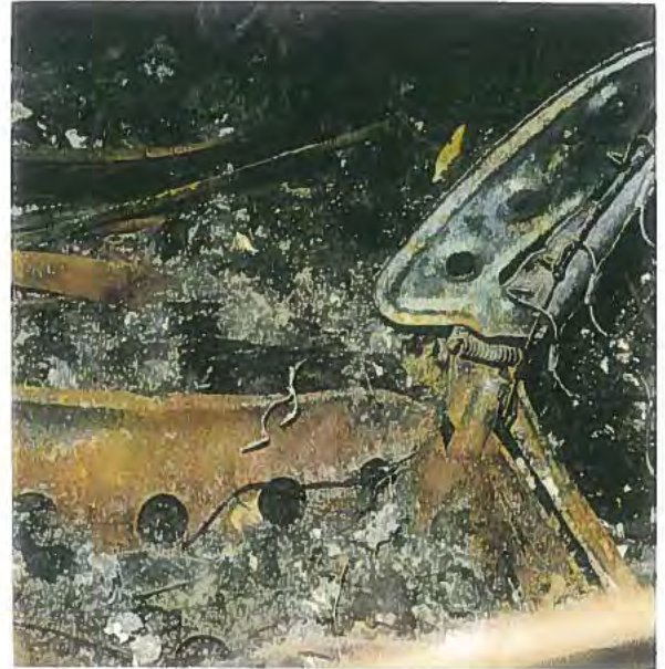
IB REAR CORNER OF SEAT PAN BUCKLED - LATERAL CONTACT W/ TUNNEL
