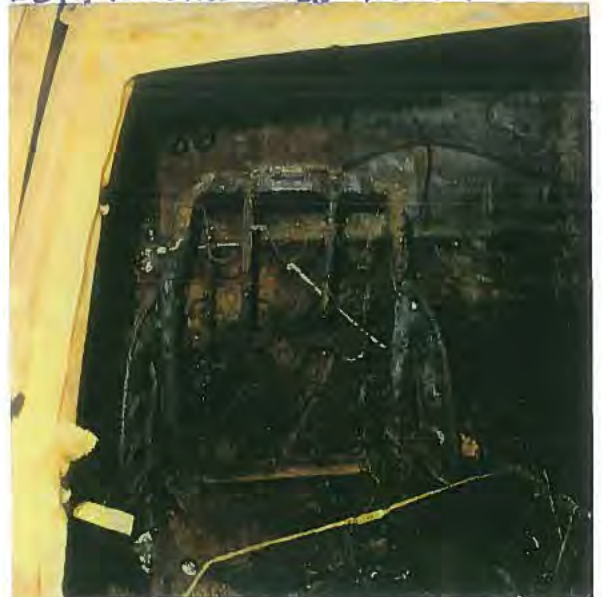
RF SEAT IB WING BENT IN SEAT ATTACHED SILL 3.2 NOSE UP SOLID TO VEHICLE SEAT BACK ALMOST VERTICAL
