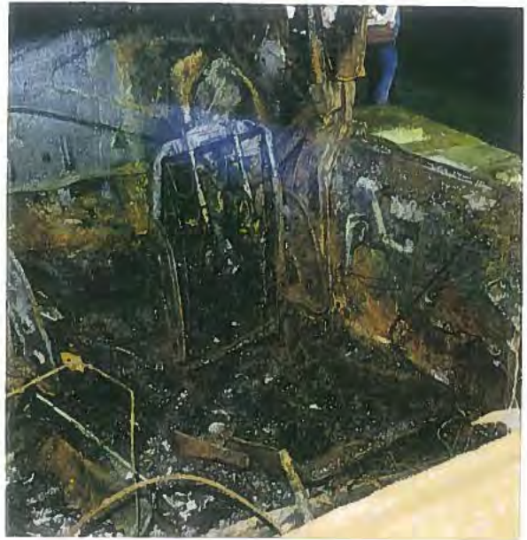
DRIVER SEAT OB SIDE OF SEAT BACK PUSHED LATERALLY IB FROM B-PILLAR CONTACT PL-02
