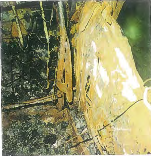
ADJ PIN PUT DENT IN B-PILLAR SURFACE
