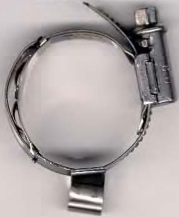
Properly Torqued Clamp
