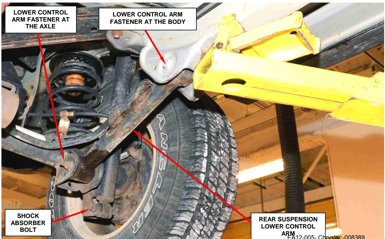
Figure 2 – Rear Suspension Lower Control Arm and Shock Absorber Fasteners
