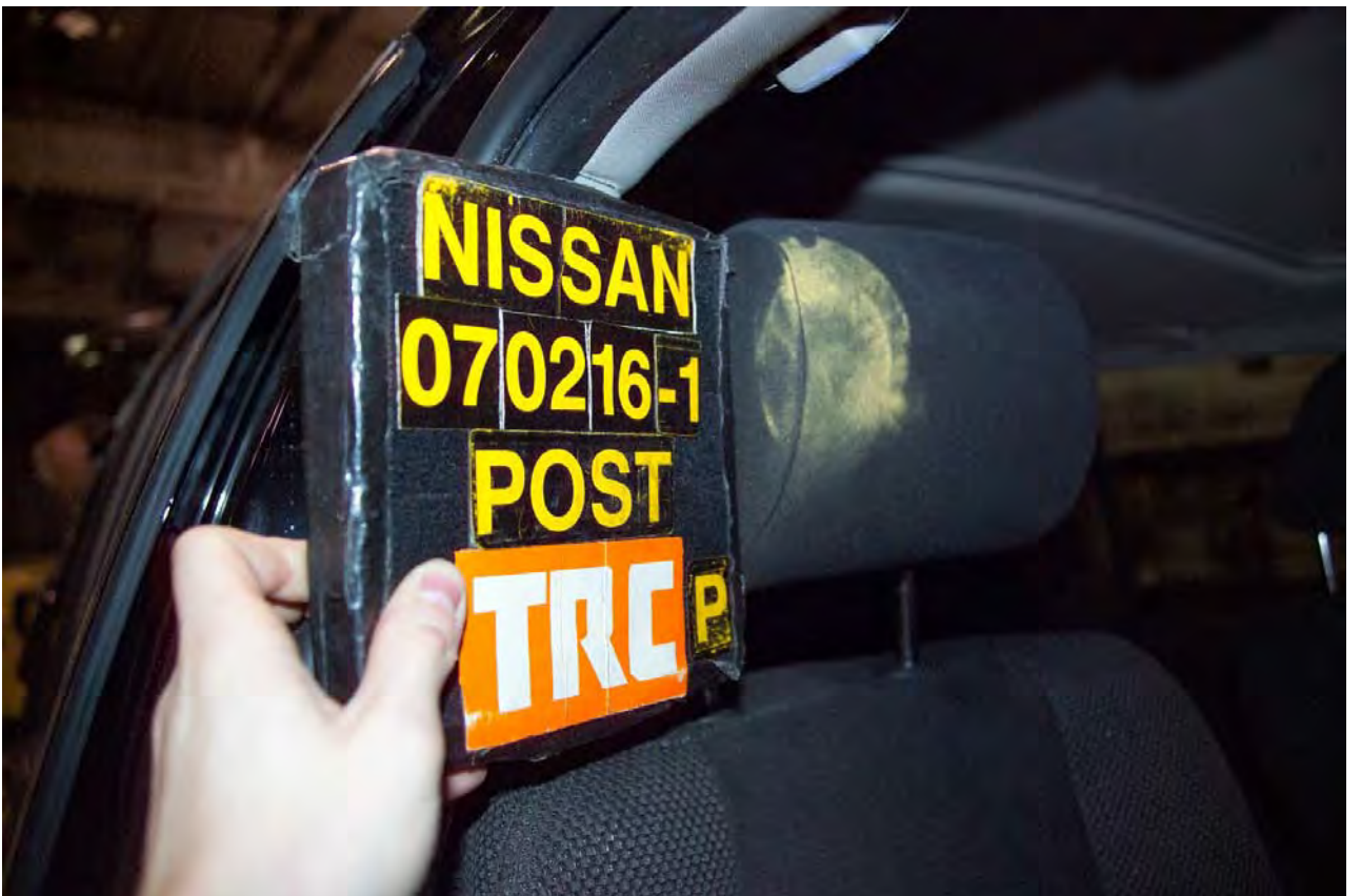
Figure A-46 Post-Test Passenger Rebound Chalk Mark View
