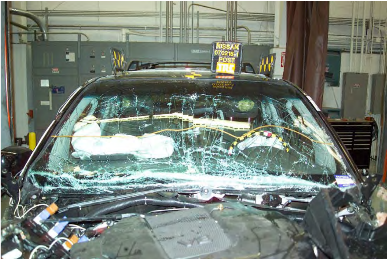
Figure A-59 Post-Test Windshield Front View (Hood Removed)
