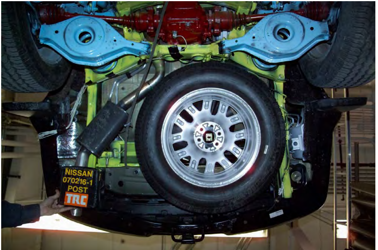
Figure A-24 Post-Test Under Floor - Rear (View 5)
