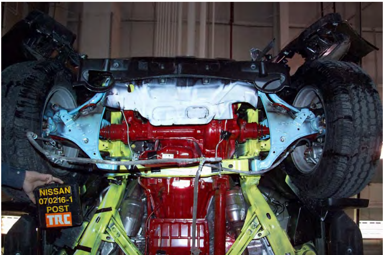
Figure A-16 Post-Test Under Floor - Front (View 1)
