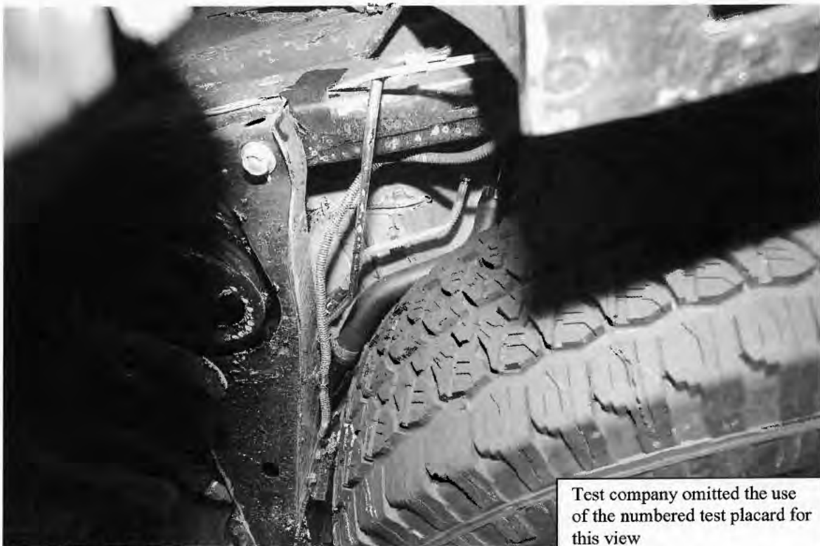
Photo No. 20 POST-TEST Subject: Filler Hose View
