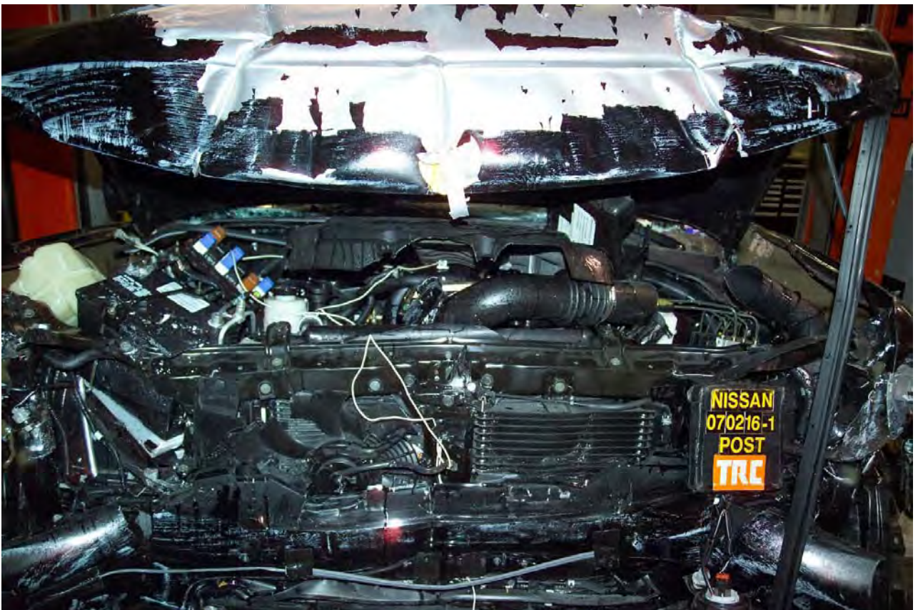
Figure A-61 Post-Test Engine Compartment Plan View (Hood Removed)
