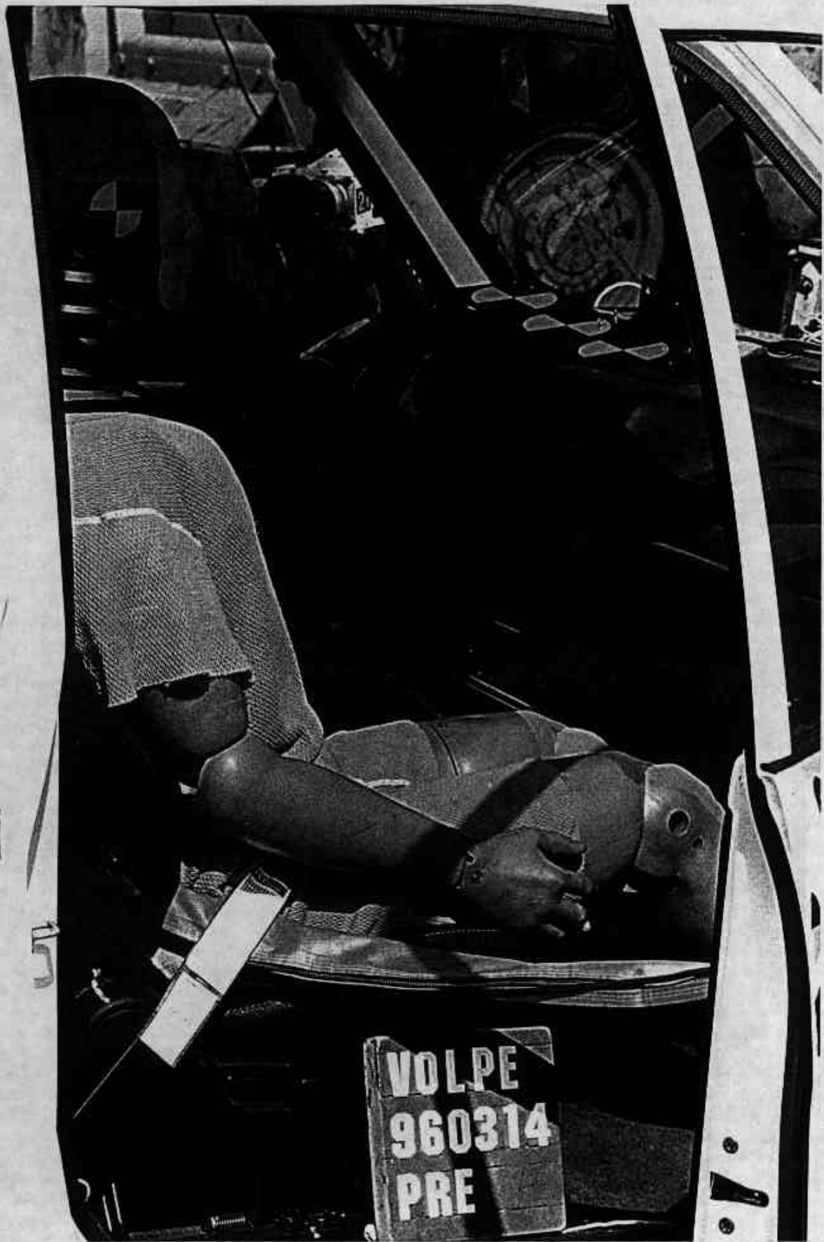
Figure A-36 Pre-Test Passenger Dummy & Vehicle Interior - View 2
