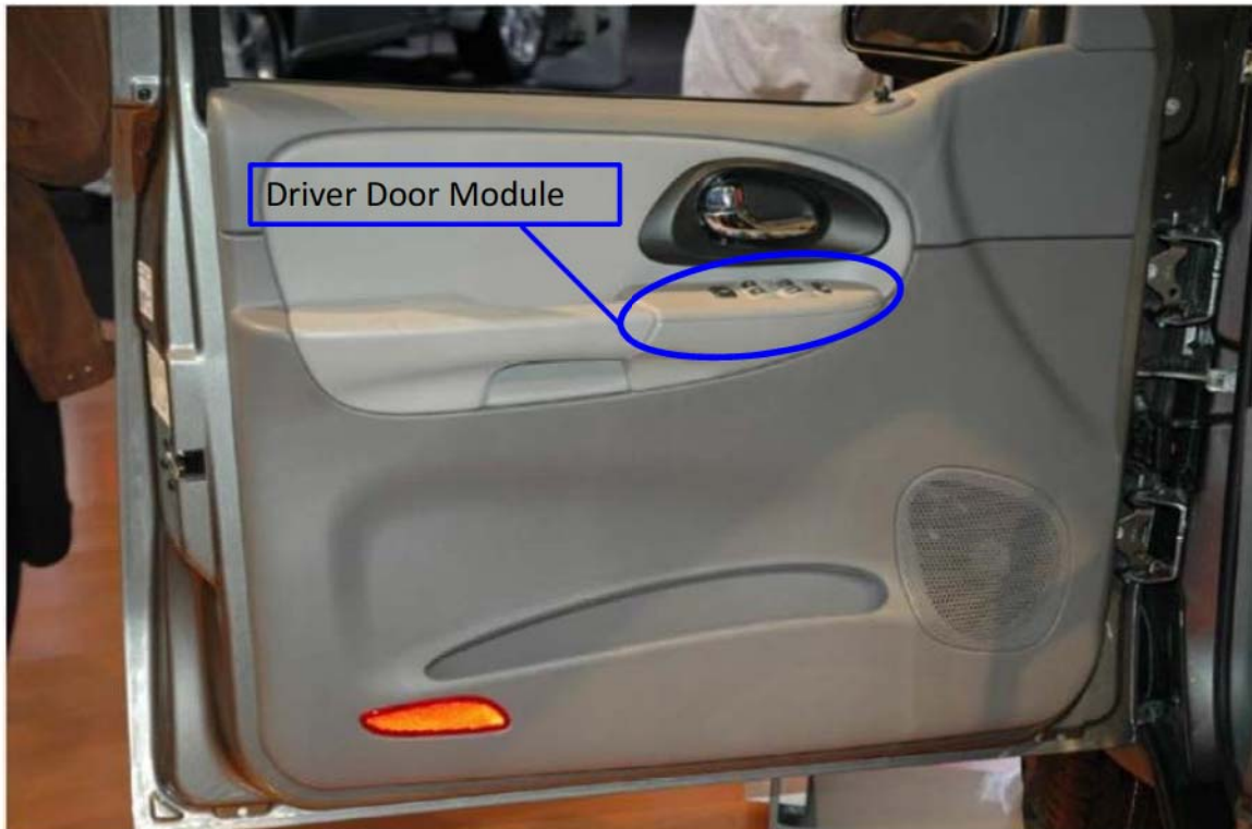
Figure 1 – Trailblazer door trim with DDM indicated.
