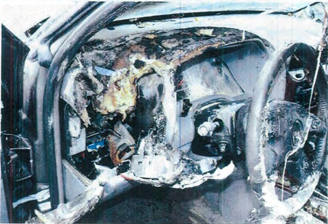
34. An overall view of the fire extension to the left side of the dashboard.
