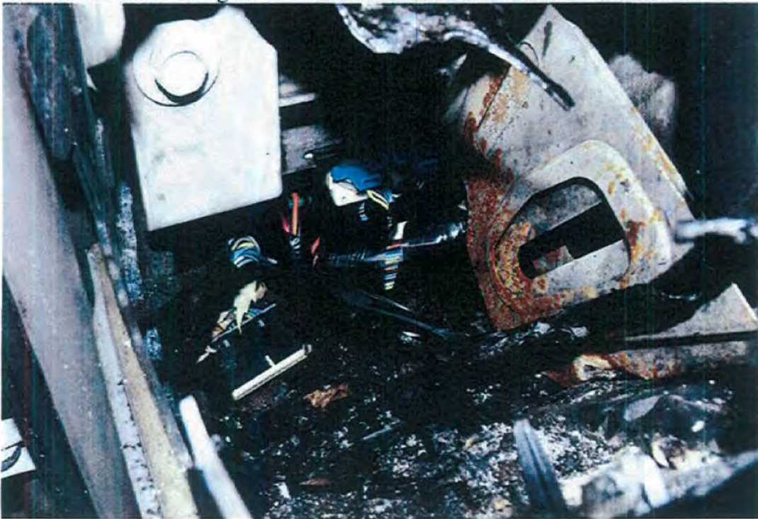
24. A view of the wiring inside the dashboard on the left or driver's side intact.
