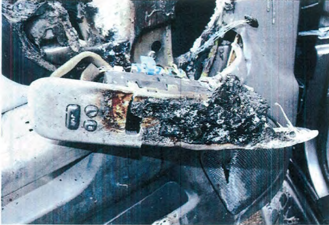
27. A view of the driver's door control panel removed.
