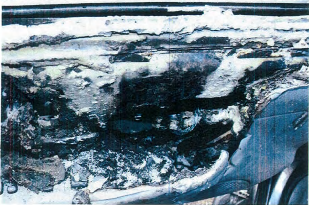
26. A view of fire damage within the driver's door panel.
