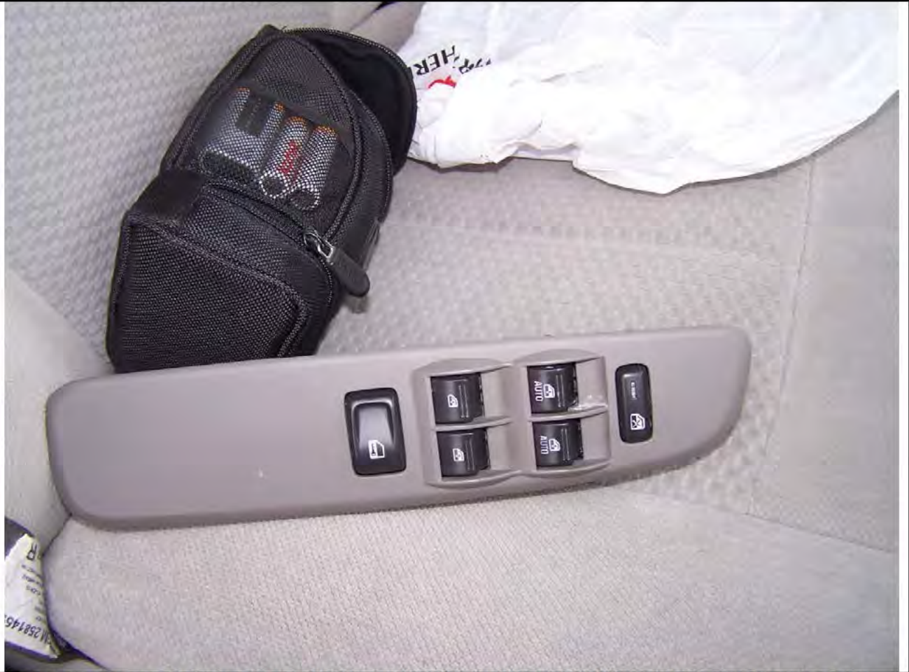
970 ON SIDE OF LEFT FRONT DOOR MASTER SWITCH SHOWING DEFORMED AREA NEAR LEFT END.
