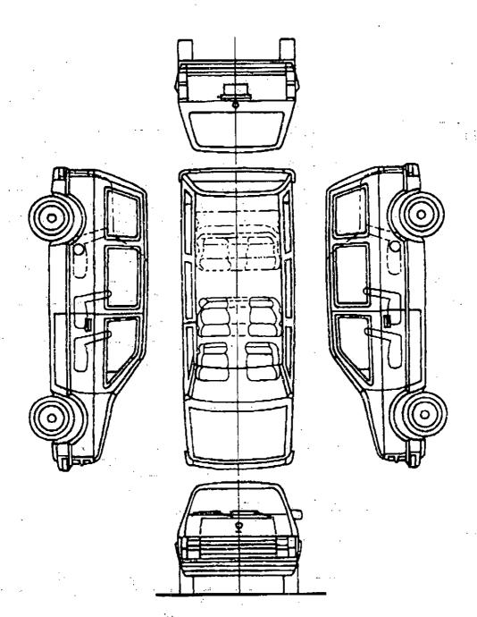
Sketch damage on all views. Include dimensions to describe and locate each damaged area and maximum depth of penetration for each impact. Annotate observations which might be useful in reconstructing the accident (e.g., direction of scrapes, markings on tires and wheels, etc.). Take photographs.
