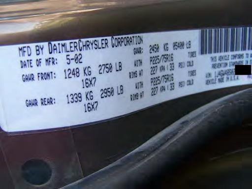
THIS VEHICLE CONFORMS TO ALL APPLICABLE FEDERAL MOTOR VEHICLE SAFETY AND THEFT TIRES DATE OF MANUFACTURE SHOWN ABOVE. PREVENTION STANDARDS PS1) COLD TIRES TRIM: E7L5 UEHICLE MADE IN U.S.A. PSI) COLD
