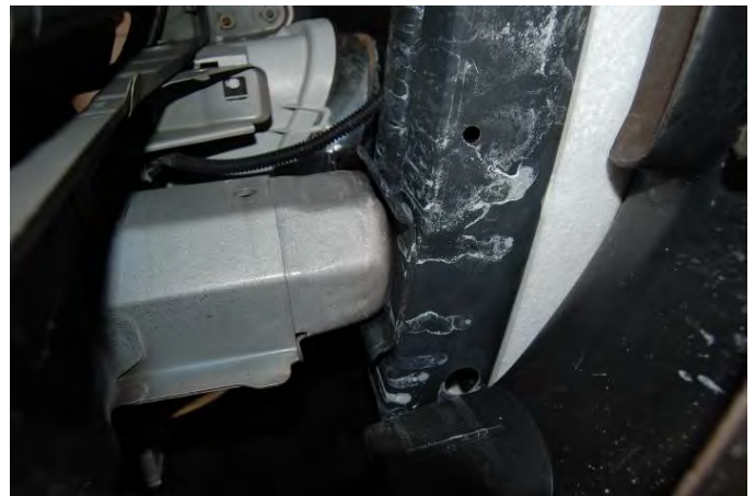
Left frame rail and bumper support – no damage
