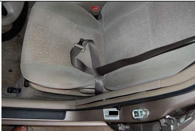
Driver side pretensioner deployed
