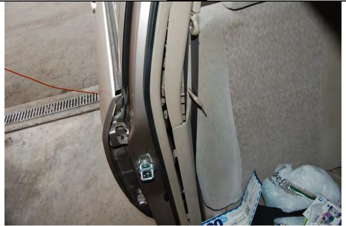
Passenger side seat belt pretensioner deployed
