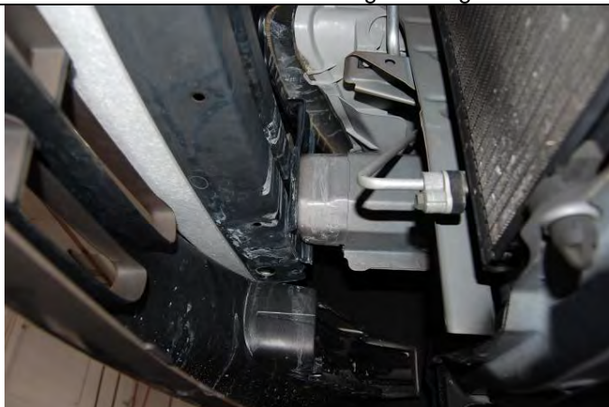
Right frame rail and bumper support – no damage
