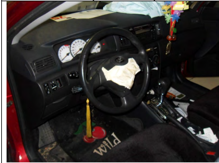
Both Front Air Bags Deployed
