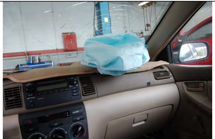
Passenger bag deployed – windshield broken
