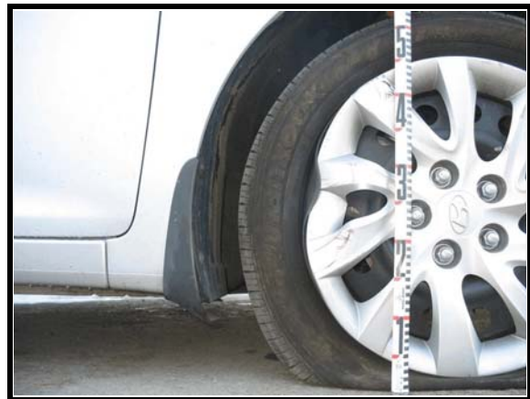
Figure 6. 2012 Hyundai Elantra, right front rim damage
