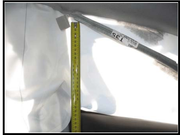
Figure 10. Stiffener position just forward of B-pillar
