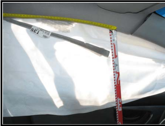
Figure 9. 2012 Hyundai Elantra, left IC air bag metal stiffener
