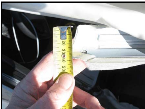
Figure 11. Forward end of metal stiffener
