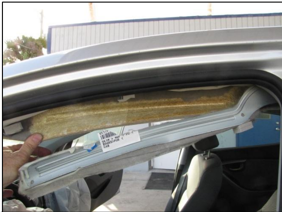
Figure 7. View from the exterior of the partially separated headliner reinforcement into the driver's compartment.
