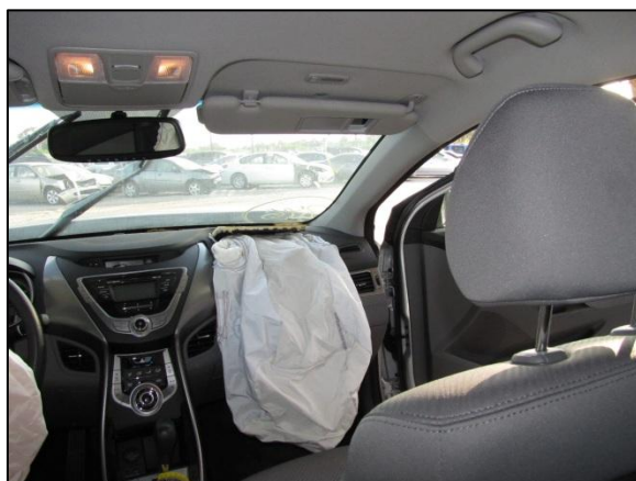
Figure 6. Deployed front right air bag of the Hyundai.
