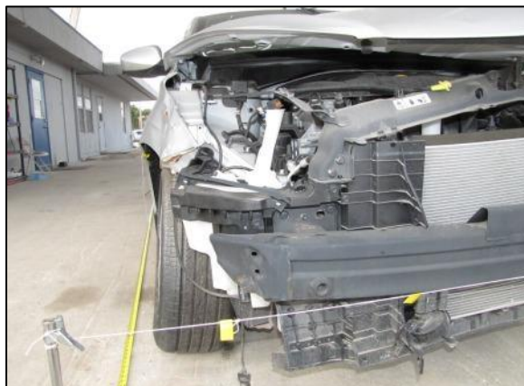
Figure 3. Front right damage to the Hyundai.
