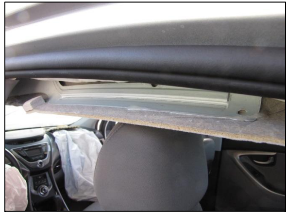
Figure 8. Exterior view of the back half of the reinforcement still attached to the headliner over the second row left position.
