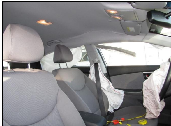
Figure 9. Partially separated headliner reinforcement against inside surface of the left IC air bag.
