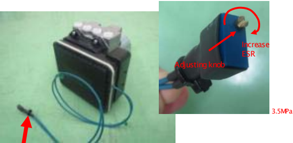
ESR adjusting knob for tantalum capacitor (PSVCC)
