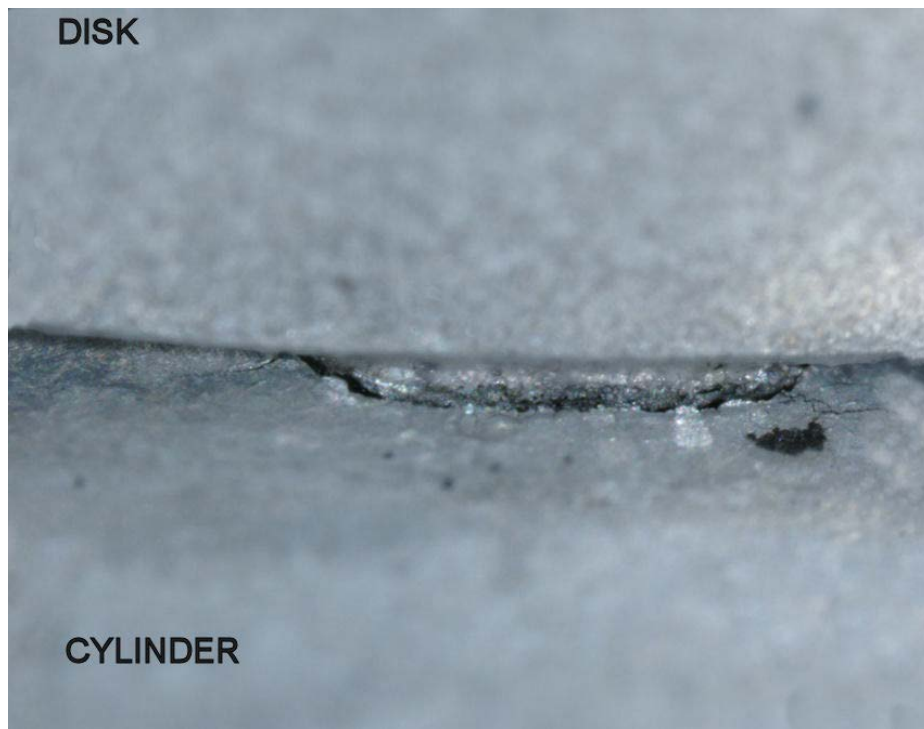
Photo 3 – The ATF cooling cylinder fracture at 25x magnification
