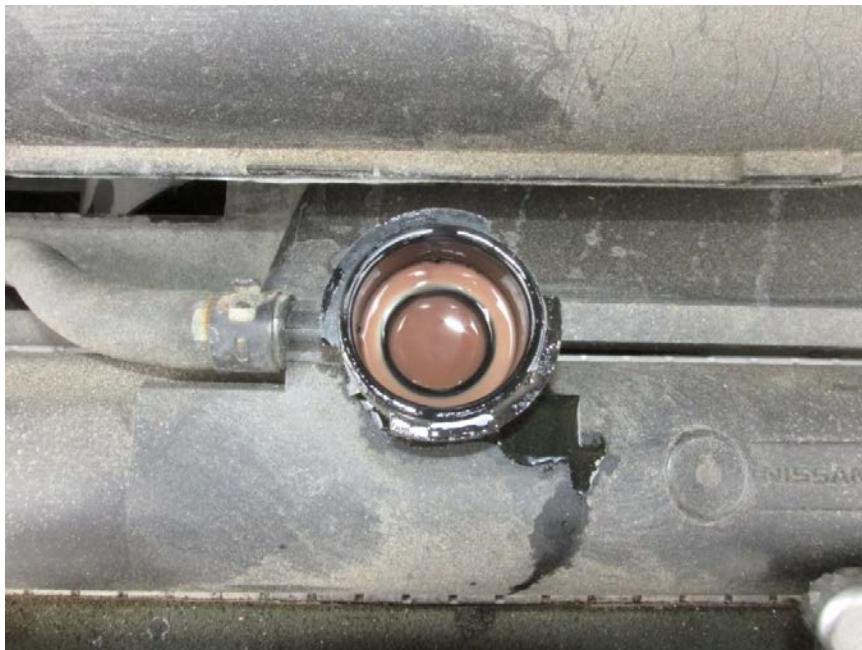
Photo 10 – June 30, 2016 - 2005 Xterra - co-mingled ATF/Coolant
