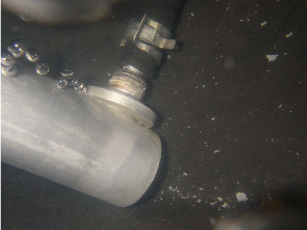
Photo 2 – Leak at left ATF port from submerged cooling cylinder
