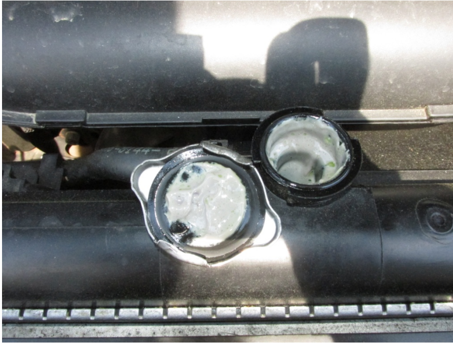
Photo 8 – June 30, 2016 - 2006 Pathfinder - co-mingled ATF/Coolant
