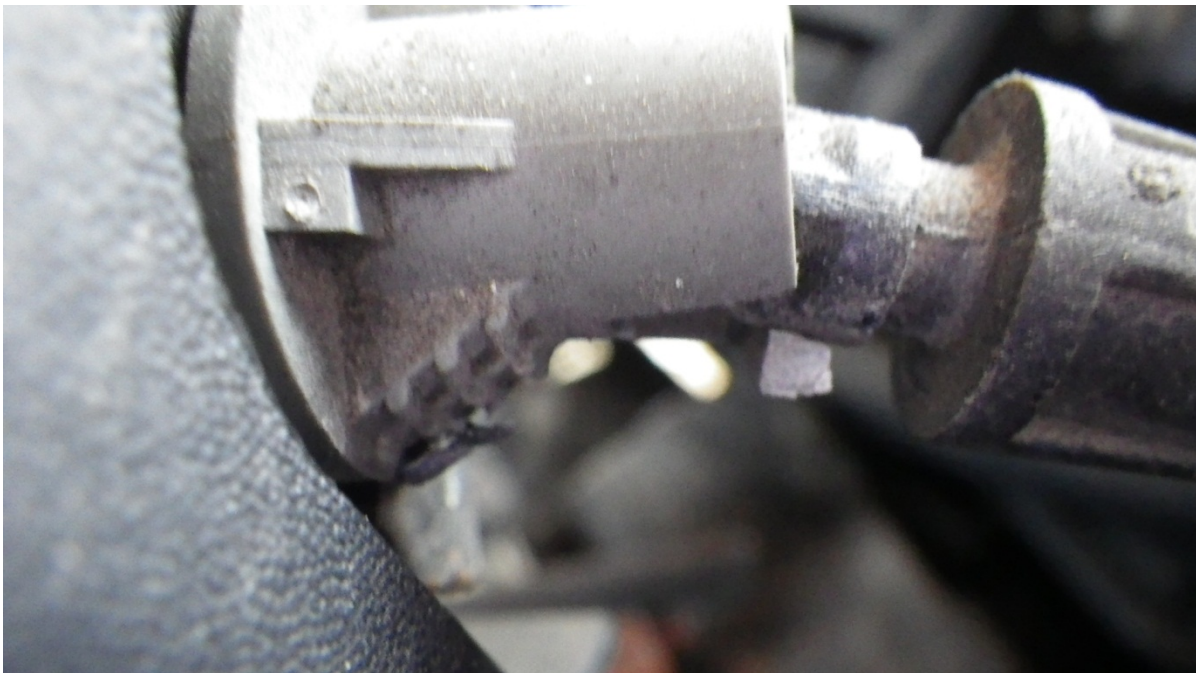
Figure 4. Fractured collar tab with unretained ferrule, side view.
