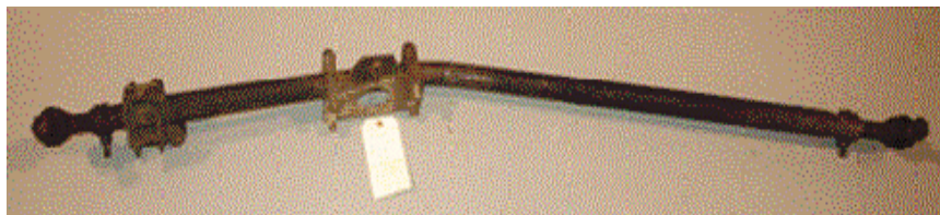
Figure 55- Greyhound 6352 Signature Bent Tie Rod
