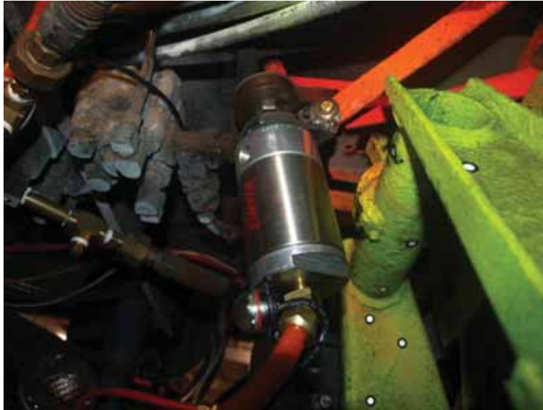
Figure 14- Caster Latch Tongue Lift Cylinder
