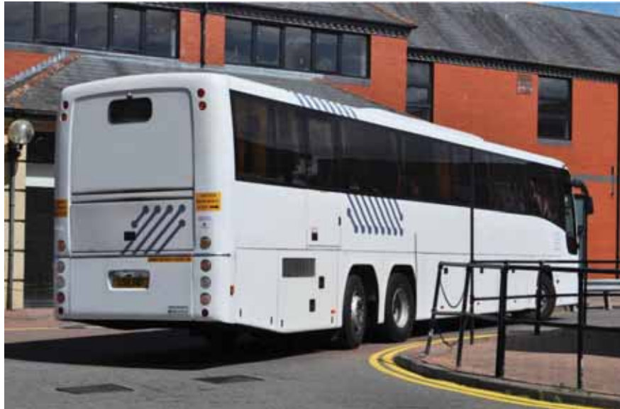
Figure 1 - Motor Coach Shown Turning with Steerable Rear Tag Axle
