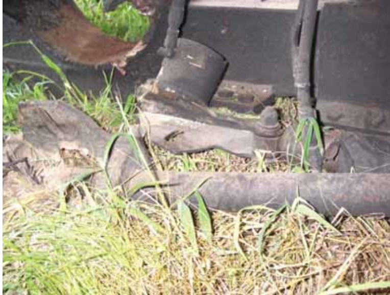
Figure 37- Greyhound 6352 Impact Damaged Tie Rod and Latch
