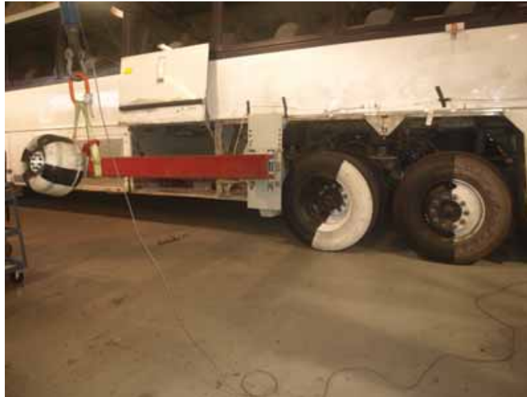
Figure 20- Vehicle Outriggers Undergoing Integrity Load Test
