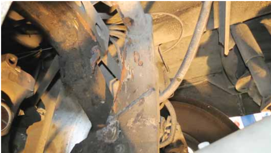
Figure 29- Americanos 60630 Impact Damage to Tag Axle Caster Arms
