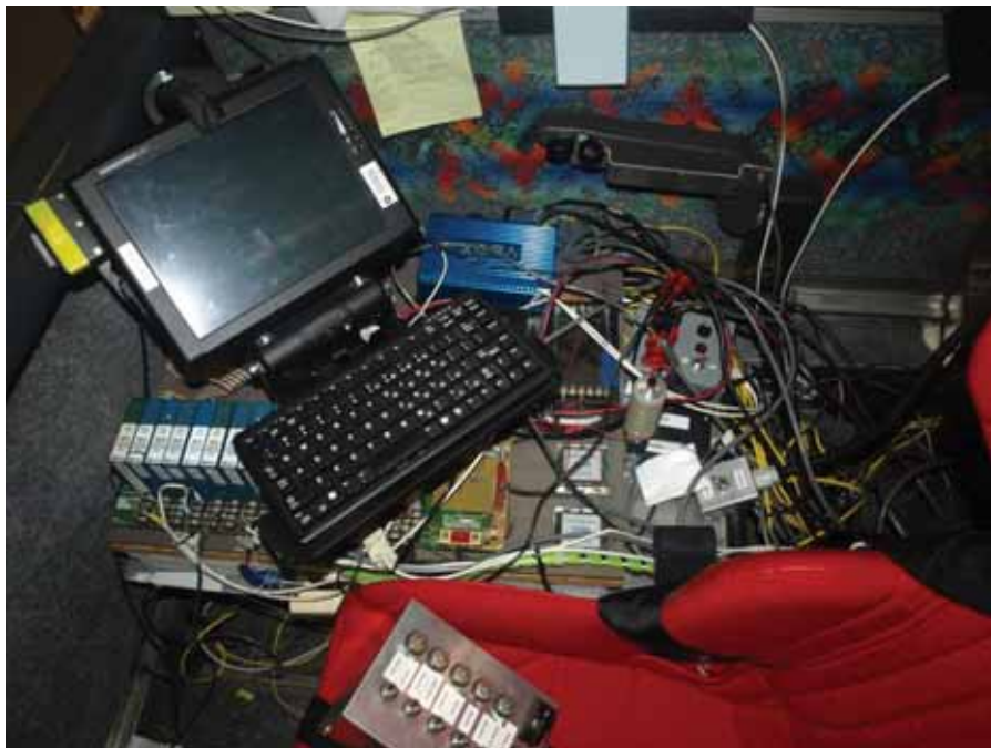
Figure 17- Instrumentation Data Acquisition Package
