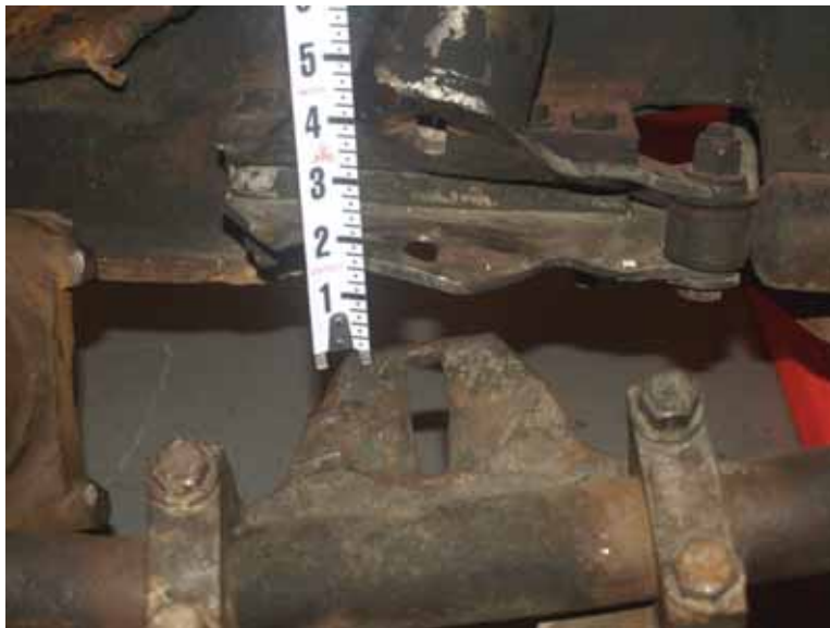
Figure 66- Greyhound 6352 Separated Tie Rod Latch Plates
