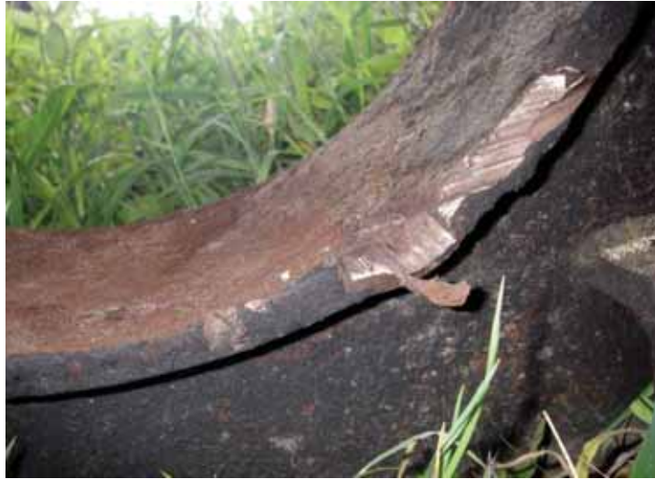
Figure 39- Greyhound 6352 Impact Damage as Driveshaft Escaped Pass-Through
