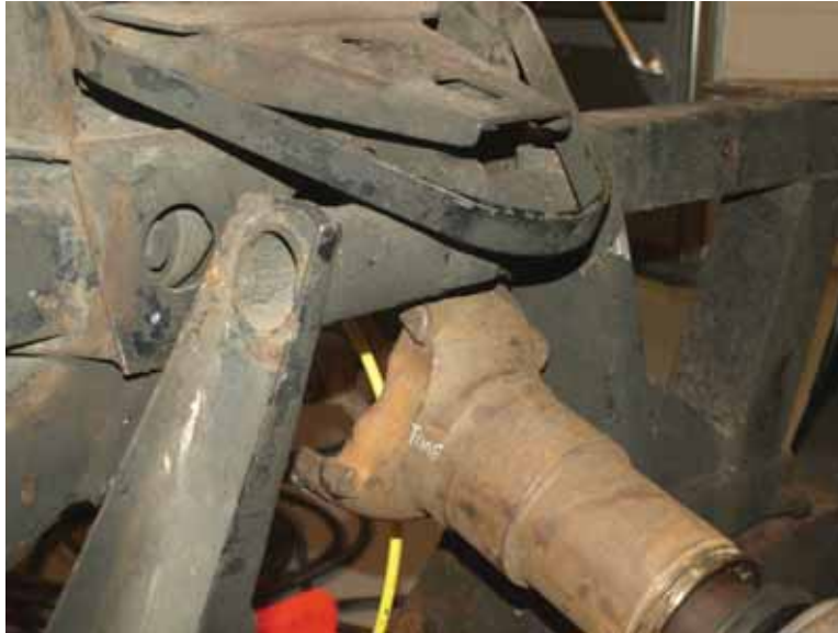
Figure 67- Greyhound 6352 Illustrating Impacting Caster Latch Arm Assembly
