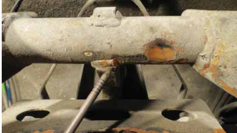
Figure 62- Americanos 60630 Heavy Impact Damage to Caster Latch Arm
