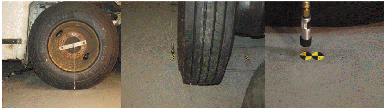
Figure 68- Measuring Caster Angle Change on VRTC Bus Using Lasers
