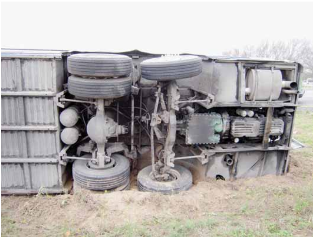
Figure 27- Americanos 60630 Crash Scene Bent Tie Rod
