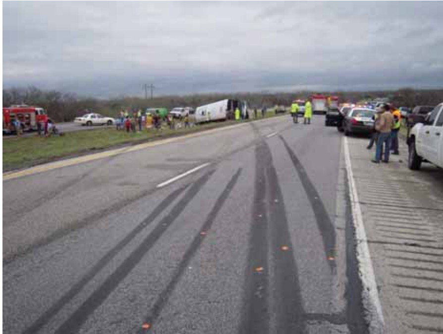
Figure 24- Crash Scene Tire Markings
