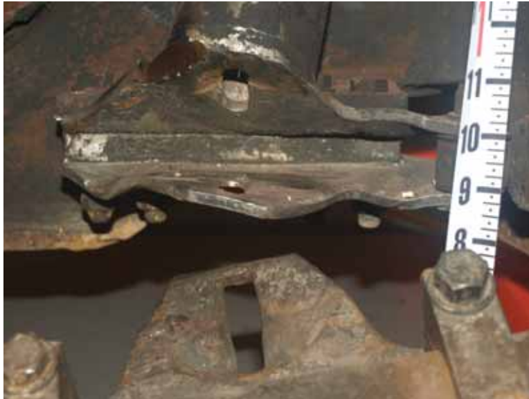
Figure 58- Greyhound 6352 Defeated Tag Axle Tie Rod Latch
