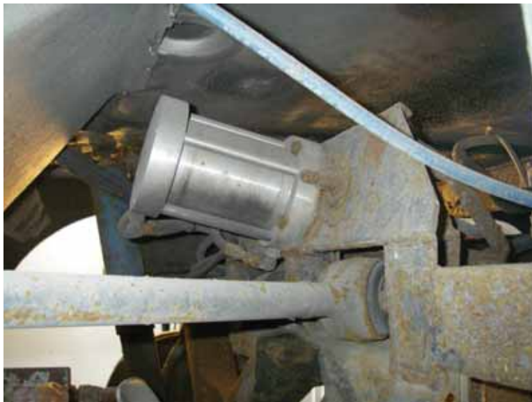
Figure 9- Auxiliary Controlled Caster Position Cylinder
