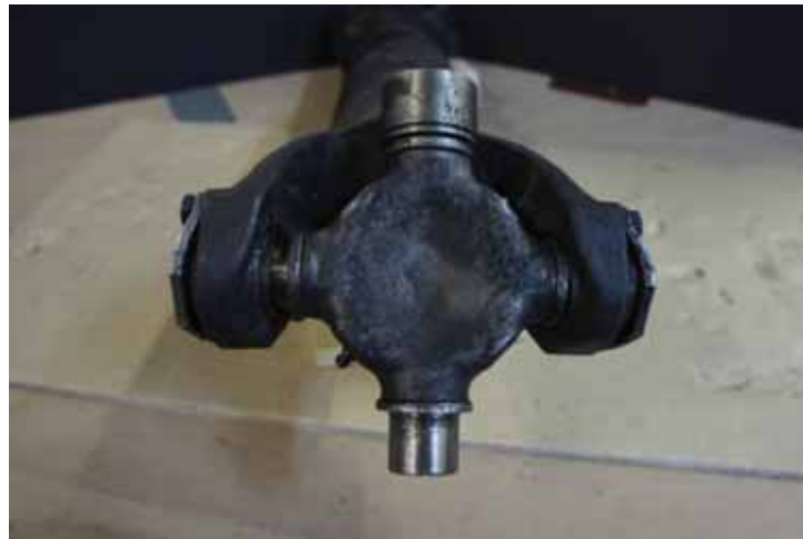
Figure 52- Greyhound 6352 Drive Axle U-Joint Overload
