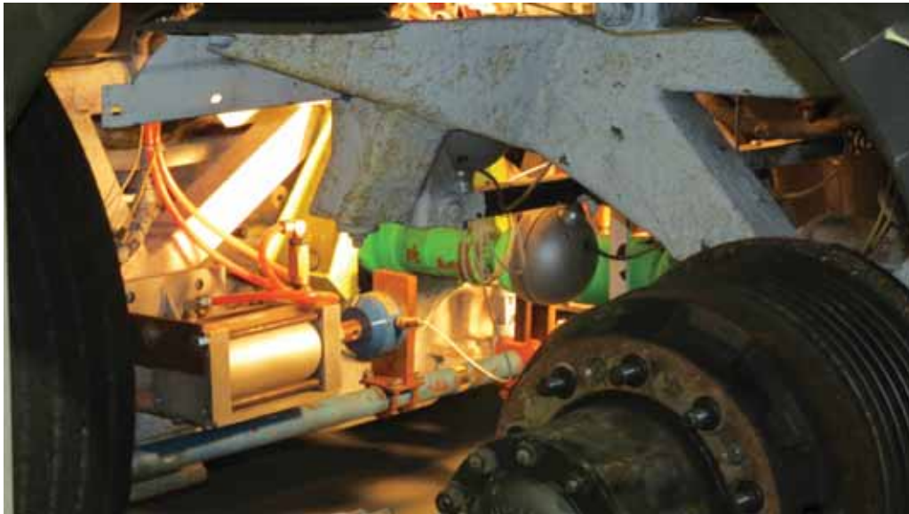
Figure 13- Tie Rod Push Cylinder
