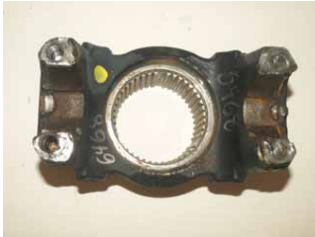
Figure 47- Greyhound 6468 Transmission Hub Damage
