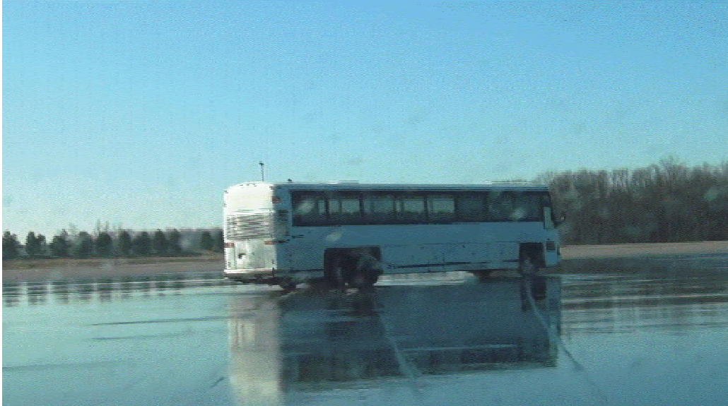
Figure 77- VRTC Bus Tag Axle Steering with Reversed Caster Test
