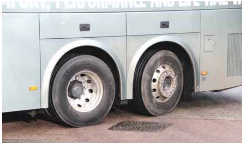
Figure 2 - Steerable Rear Tag Axle with Wheels Turned
