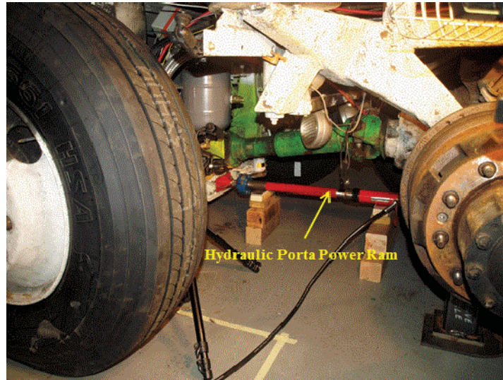
Figure 72- Loading Axles on VRTC Bus with Hydraulic Ram
