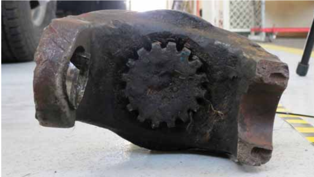
Figure 32- Americanos 60630 Over-Compressed Driveshaft
