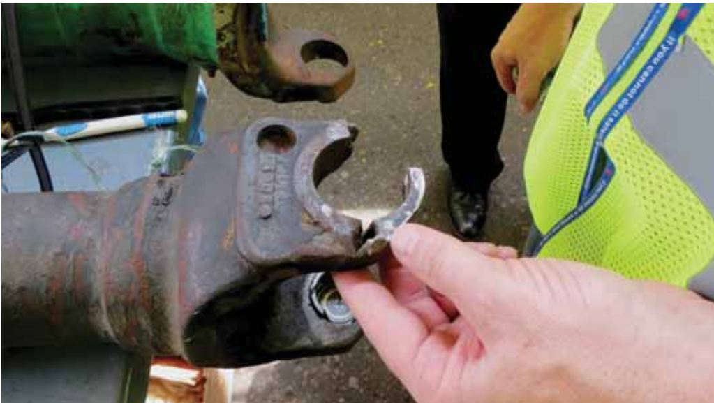
Figure 31- Americanos 60630 Driveshaft Fractured Piece Mate
