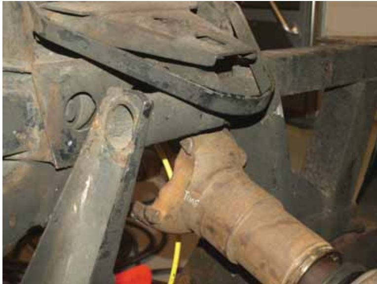
Figure 61- Greyhound 6352 Arrangement of Components that Affect Latching Tongue
