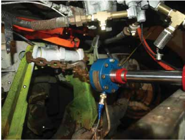
Figure 69- Pulling Caster Arms to Safety Catch on VRTC Bus
