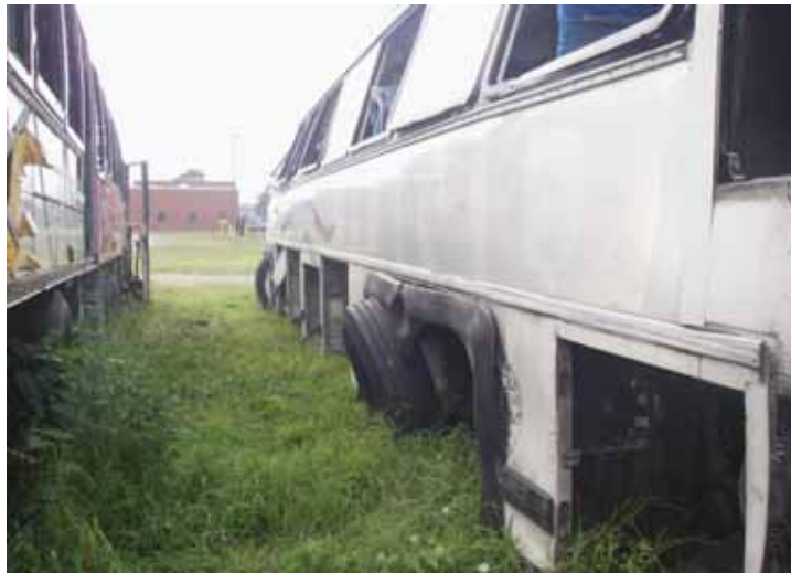
Figure 40- Greyhound 6352 Deflated Outside Drive Tire Damage
