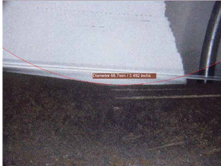
Figure 41- Greyhound 6352 Tie Rod Impact Radius Measurement
