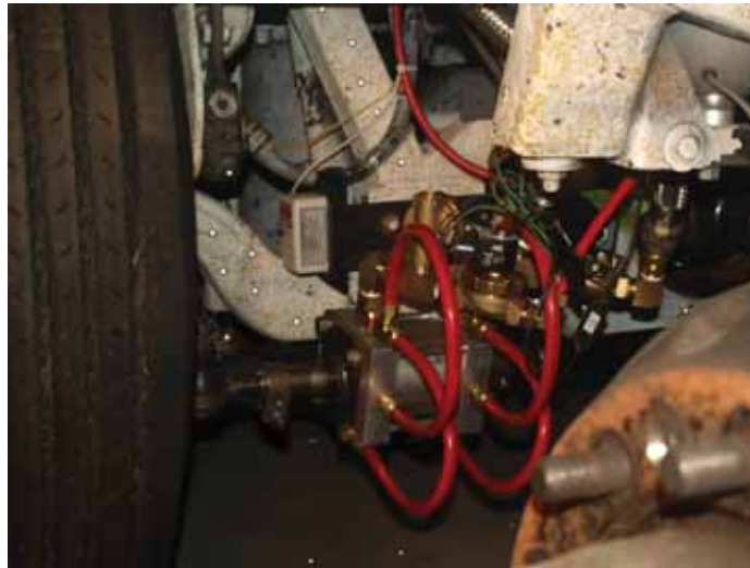
Figure 15- Fast Action Pneumatic Toe-in Tie Rod Installed
