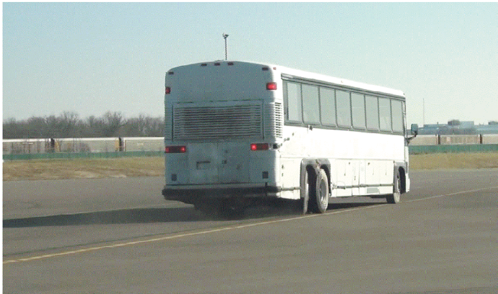
Figure 76- VRTC Bus Forced Tag Axle Steering Trial Testing
