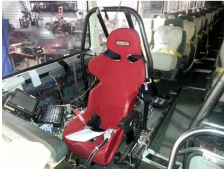
Figure 7- Water Dummy Ballasted Seats
