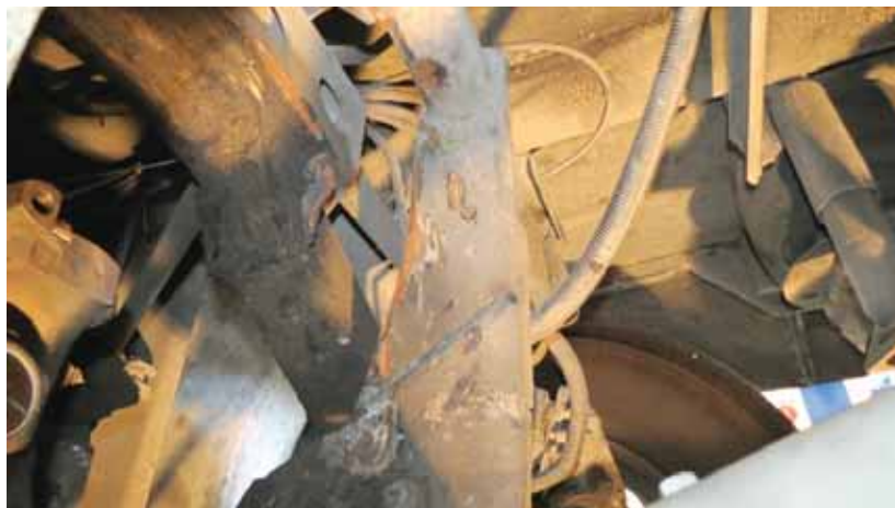
Figure 59- Americanos 60630 Caster Arm Levered Into Negative Caster by Driveshaft
