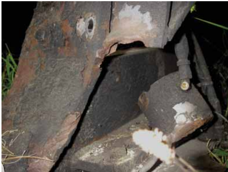
Figure 38- Greyhound 6352 Impact Damage to Tag Axle Caster Arms
