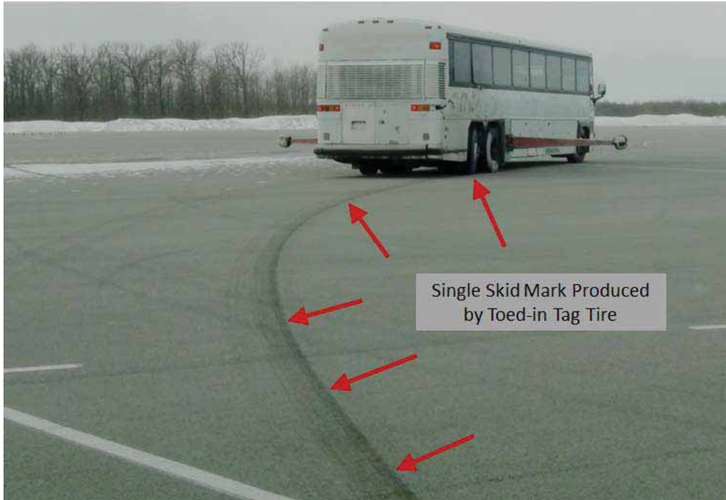
Figure 79- VRTC Test Vehicle Replicating Accident Single Tire Marking
