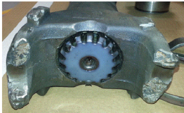
Figure 48- Greyhound 6468 Fractured Cast Journal Ear
