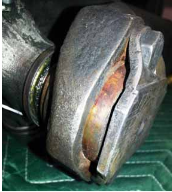
Figure 53- Greyhound 6352 Deformed Bearing Retainer Plate
