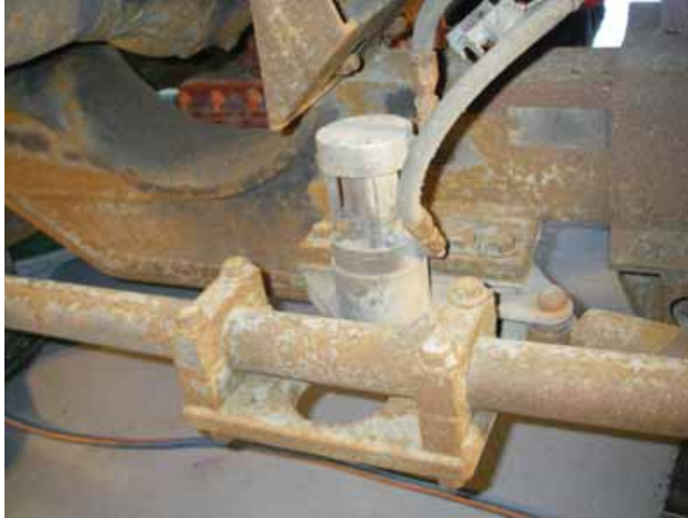
Figure 10- Auxiliary Controlled Tie Rod Latching Cylinder
