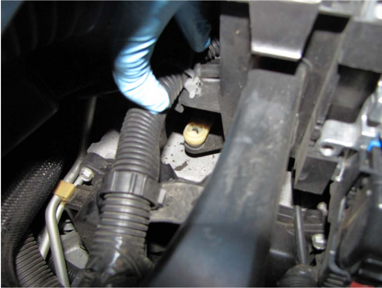
1565 VIEW OF TRANSAXLE SHIFT CABLE
