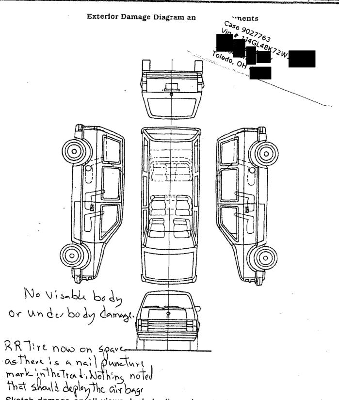
Sketch damage on all views. Include dimensions to describe and locate each damaged area and maximum depth of penetration for each impact. Annotate observations which might be useful in reconstructing the accident (e.g., direction of scrapes, markings on tires and wheels, etc.). Take photographs.
