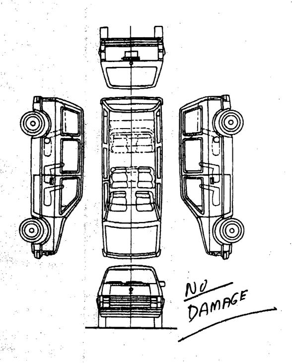
Sketch damage on all views. Include dimensions to describe and locate each damaged area and maximum depth of penetration for each impact. Annotate observations which might be useful in reconstructing the accident (e.g., direction of scrapes, markings on tires and wheels, etc.). Take photographs.
