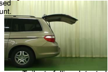
Tailgate falling detected, tailgate raised by motor.
